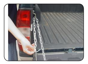
Step 3: Secure the ramp to the vehicle using the safety chain. After the safety chain is secure, test the ramp by pulling backwards on it. Make sure it does not slide back or disengage from the loading surface.
