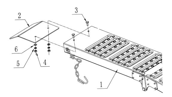
Step 1: Unfold the tri-fold ramp, assemble the lip to the ramp.
