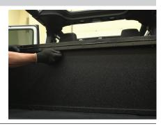
With the center section attached, lift and fold the lid section over to the back seat.
