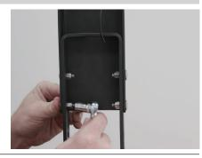
Lay the factory spare tire carrier on a flat surface and remove the four T-25 torx screws securing the light to the housing.
