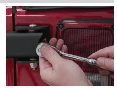
Remove the hex head hinge bolt used to align the hinge to the door and open the hinge 90°. Fully tighten the two inside hinge bolts to 19 ft.-lbs.
