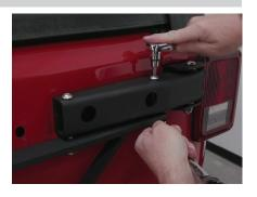
Repeat step 6 to remove the lower factory door hinge. Loosely install the lower HD replacement hinge following step 7.
