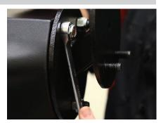
Lift the spare tire back onto the three mounting lugs and secure with the factory lug nuts.
