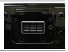
To install the new support brackets, the factory weld nut must be removed.
