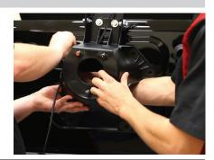
With the 8mm fasteners reinstalled, completely tighten all the hardware.
