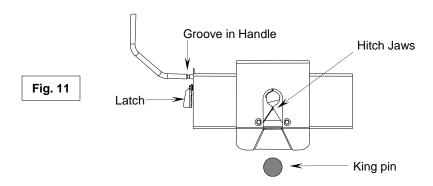
4. With handle in the closed position (See Fig. 11), back truck slowly into trailer. As the trailer king pin enters the hitch it will push the hitch jaws open and extend the handle (See Fig. 12). As king pin completely enters head, jaws will spring closed around king pin and handle will return to the closed position. (See Fig. 13)
