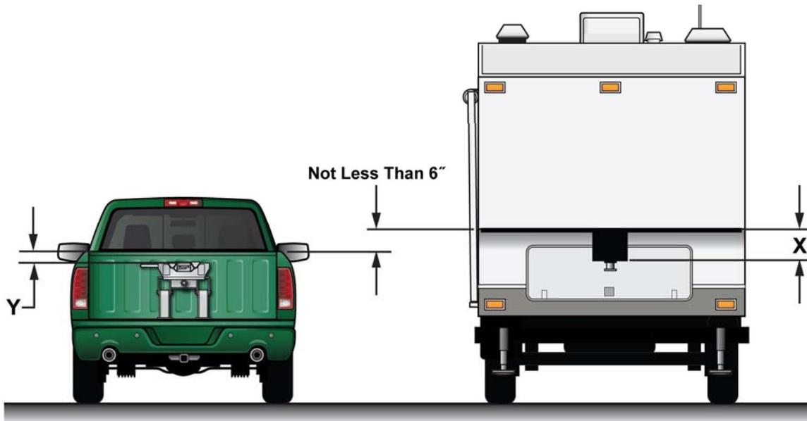
2. With top face of head level measure up to top of pickup box (dimension Y in Figure 1). On the trailer measure up from the face of the pin box to the underneath of the trailer (dimension X in Figure 1). Measurement X less measurement Y gives the amount of clearance between the top of the pickup box and the underneath of the trailer. At a minimum this should be 6", if the trailer and tow vehicle are going off-road then this needs to be 8" to 10".
