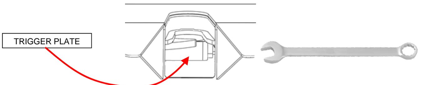
Using a WRENCH, (Keep fingers out of Jaw area) press on the Trigger Plate located underneath the Jaw. Pressing on the Trigger Plate will release the jaw mechanism and it will fully close. The Lock Hasp Indicator should now show that the Jaw is closed.
