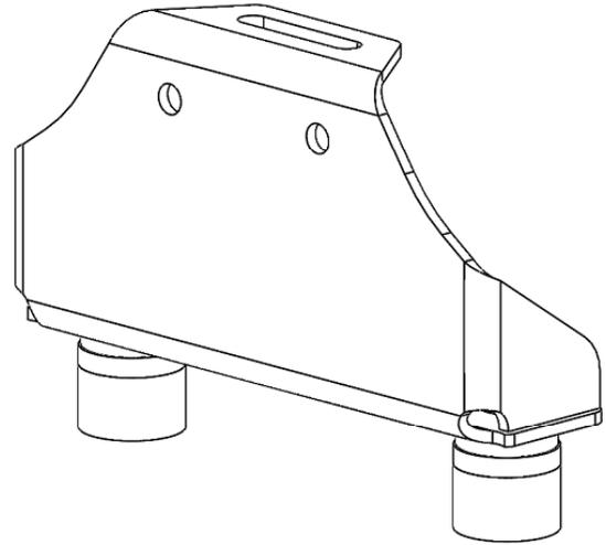
3. Install the cross member from kit 32998 or 32999 to uprights (#1) using the  $\frac{3}{4}$ "-10 bolts (#8) and  $\frac{3}{4}$ "-10 nylock nuts (#9). Kit 32998 shown below as an example; kit 32999 installs similarly.
