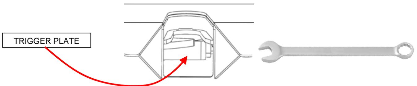
Using a WRENCH, (Keep fingers out of Jaw area) press on the Trigger Plate located underneath the Jaw. Pressing on the Trigger Plate will release the jaw mechanism and it will fully close. The Lock Hasp Indicator should now show that the Jaw is closed.
