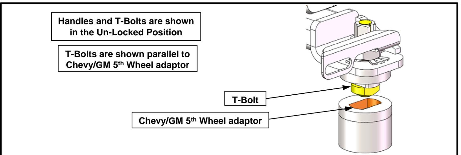
2. Once uprights are installed; turn handles into the locked position. This may require adjusting the T-bolts for a looser or tighter fit.
