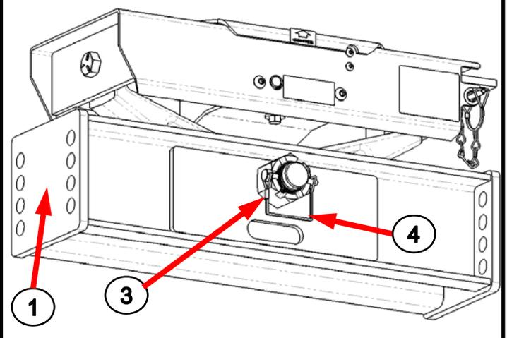
5. Using a grease gun, grease Zerk fitting on plate side of pivot pin
