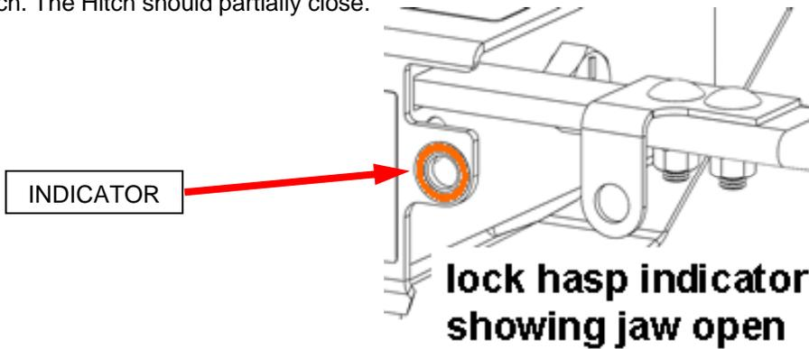
Looking on the back of the Hitch, the indicator should be as shown in the sketch.
