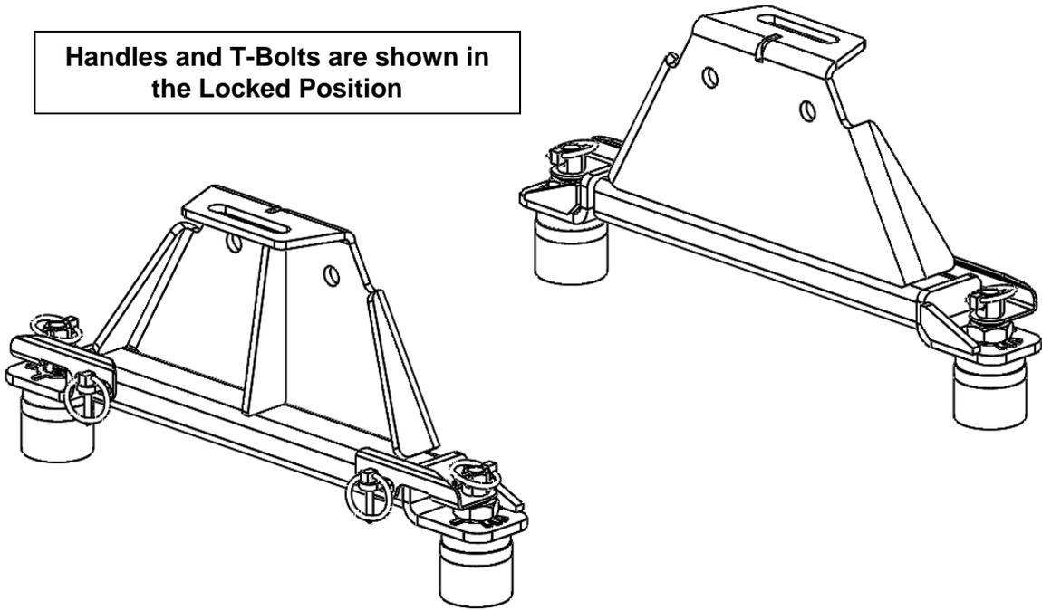
3. Install the cross member from kit 32998 or 32999 to uprights (#1) using the  $\frac{3}{4}$ "-10 bolts (#9) and  $\frac{3}{4}$ "-10 nylock nuts (#10). Kit 32998 shown below as an example; kit 32999 installs similarly.
