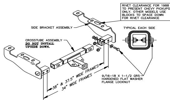
1. REMOVE PICKUP TRUCK SPARE TIRE AT END OF FRAME FROM ITS UNDER BED MOUNTING. THIS IS NOT REQUIRED FOR EACH INSTALLATION BUT WILL MAKE RECEIVER INSTALLATION EASIER. IT IS TO BE REINSTALLED WHEN INSTALLATION IS COMPLETE.
