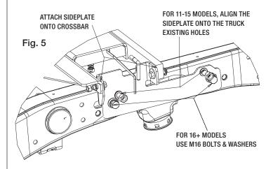
**10.** Repeat the sideplate installation on the passenger side. Tighten both driver & passenger sideplates to 80 ft-lb for 1/2" bolts and 60 ft-lb 5/8 bolts.
