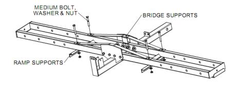
STEP 3. PLACING THE LARGE BOLTS. The carrier is designed to load the bike from the left or right side using the ramp. There are 3 sets of center boles and 1 set of upper holes on each cradle. The large safety pins and clevis pins are used in the upper holes. See FIG 5. The 4 large bolts are used in the center hole to support the bike tires. Note: Depending on
