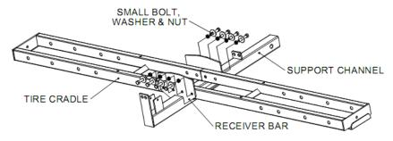
STEP 2. Attach 2 bridge supports and 2 ramp supports as shown using 4 medium bolts and nuts. NOTE: When mounting ramp supports, make sure flat surface is up and the extra 3 inches is on the outside to support the ramp while transporting.
