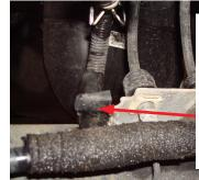
Pull left on harness to remove the "cup" from the ABS/ Brake line axle junction bracket and secure out of the way for next step.
