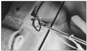
5. Leak test the inflation valve for leaks at the air line connection or dirt or debris in the valve core (Figure 22).
