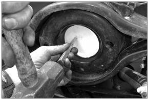
2. Center punch and drill a <sup>3</sup>/<sub>4</sub>" hole to provide valve stem clearance (Figure 6).
