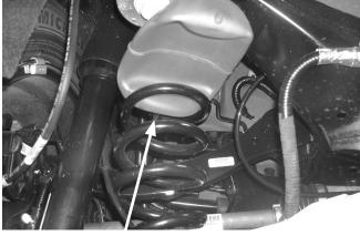
Insert cylinder with stem pointing down
