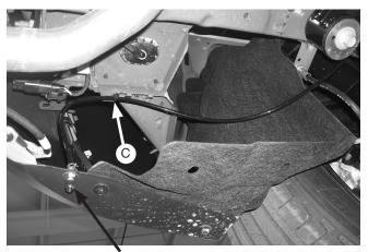
Suggested Schrader valve assembly location Fig. 9
