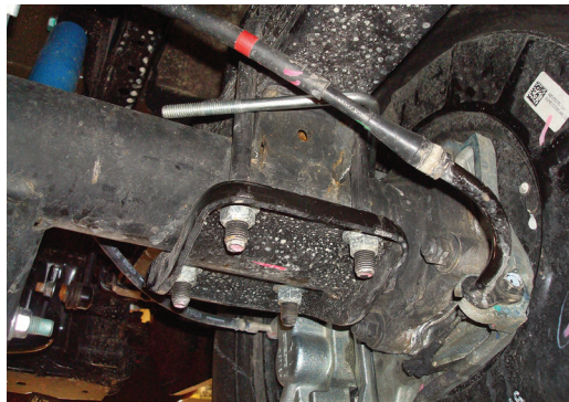
fig. D.9 Start U-bolt from the front side of the axle and rotate backward around the spring perch.
