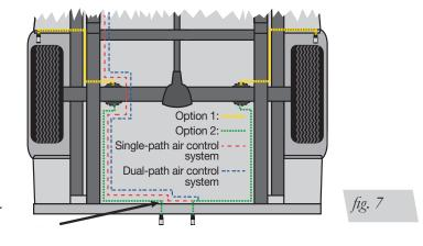
Whatever the chosen location, make sure there is enough clearance around the inflation valves for an air chuck.
