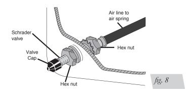
approximately 1/2" - to easily apply a pressure gauge or an air chuck (Fig. 8).
