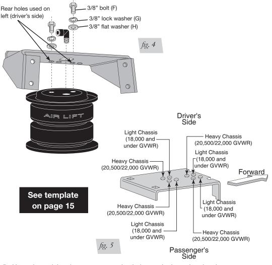
Upon determining the correct mounting holes on the lower bracket, insert two carriage bolts (J) into the lower bracket (Fig. 1). Attach the air spring assembly to the lower bracket using two 3/8" bolts (F), lock washers (G), and flat washers (H). Tighten bolts to 20 lb.-ft.
