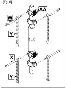
Install two (2) Lower Wheel Cradles **[X]** with Rubber Straps **[Y]** facing in <u>opposite</u> directions as shown. [Fg. 6 & 7]
