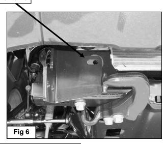
10mm x 120mm Hex Bolt 10mm x 34mm Large Flat Washer Spacer Washer
