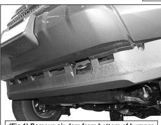
(Fig 1) Remove air dam from bottom of bumper
