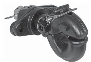
**2.** Verify pintle is in the proper coupling position as shown (latch on top).
