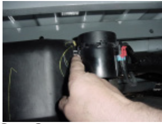
Step 2: Disengage the locking pin.
