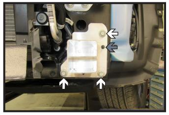
8. Using a 15MM socket, remove the three (3) bolts from the frame extension. Using a 10MM socket, remove the nut (gray) from the frame extension. Do this on both sides of the vehicle. The frame extension will not be reinstalled.
