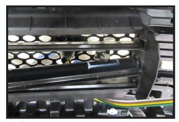
19. Shutter Models: Mark and trim shutter as shown before reinstalling. Ensure that shutters can fully open and close once reinstalled and no electrical is in the way of shutters.
