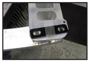
11. A spacer plate will be placed between the bumper and the frame at the top of the bumper. Before reinstalling the bumper, tape the spacer plate in position on the back of the bumper as shown.
