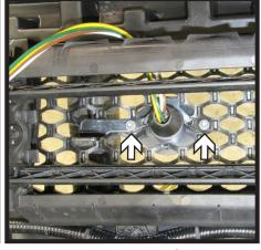
18. **Shutter Models:** Trim the fascia as shown on one side of the vehicle to allow room for the electrical (left). On the back side of the fascia remove the middle shutter to allow room to attach electrical bracket (center). Set aside shutter to be trimmed and reinstalled later. Cut a hole in the top of the shutter housing to run electrical through and install electrical bracket using two (2) 1/4" bolts with hardware (right).
