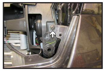
3. Using a T30 Torx, remove the two (2) bolts from the fascia, there is one (1) on each side.
