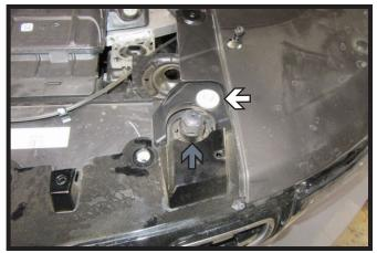
3. Using a 10MM socket, remove the one (1) bolt from the top of the fascia. Do this on both sides of the vehicle. Then turn hood bumper (gray) a quarter of a turn and remove.
