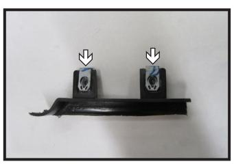
21. Remove clips from the pedestrian alert bracket and set aside to be reinstalled later.
