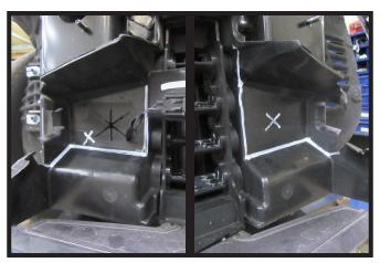
17. Using a utility knife, trim the shroud on each side of the bottom shutters as indicated.
