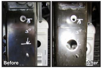
19. Measure 3" from the center of the top hole down. Using a 1-1/4" hole saw, drill hole centering hole with existing holes on the frame and the bottom of the 3" measurement. Do this on both sides of the vehicle as needed.
