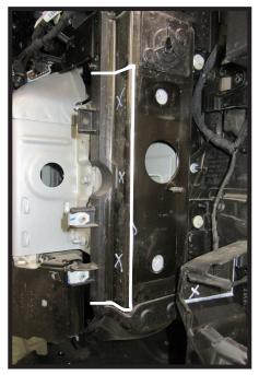
15. Using a reciprocating saw, trim the frame as shown. Do this on both sides of the vehicle.
