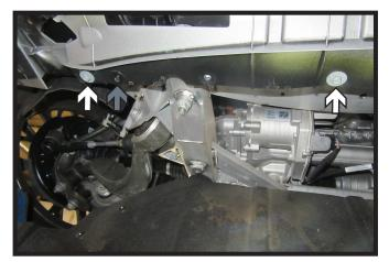
9. Using a 10MM socket, remove the four (4) bolts (white) from the underside of the fascia. Then remove the two (2) push pins (gray).
