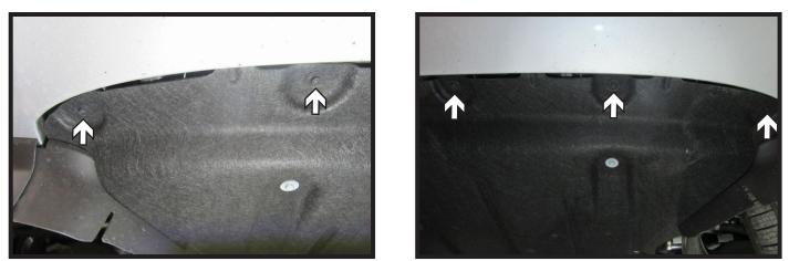
6. Using an 8MM socket, remove the five (5) bolts from the bottom of the fascia.
