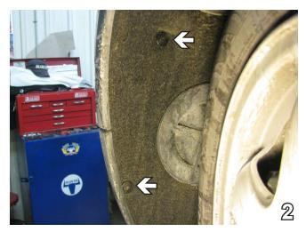
Forward the front tire, use a Phillips screwdriver to remove two (2) push pins. Do this to both sides. Set aside for later reinstallation.
