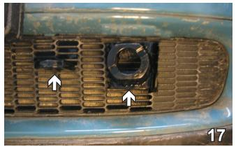
17. Reconnect the temperature sensor. Hold the fascia up to its original location. Mark and trim the fascia just on the outside edges of the receiver tube and convenience links. Do this to both sides of the vehicle. Reinstall the grill.
