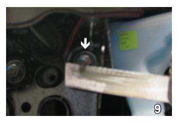
9. Use the reciprocating saw to cut off the bolt even with the nut. Do this on both sides.
