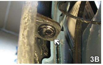
3. After removing the wheel well cover, remove two (2) push pins connecting the fascia using a flat screwdriver. Do this to both sides. Set push pins aside for later reinstallation.
