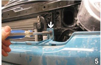
5. After removing the grill, by the headlight, there is a bolt that needs to be removed with a T25 torx. Do this on both sides. Set bolts aside for later reinstallation.
