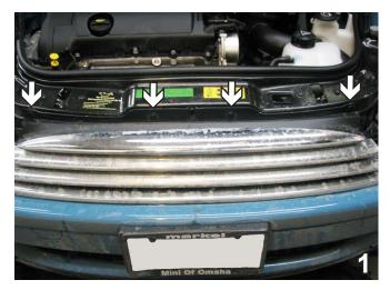
1. Using a flat screwdriver, remove four (4) push pins on top edge of grill, one (1) on each side two in the middle. Set push pins aside to be reinstalled later.
