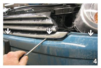
4. Remove the grill by starting from the side and working across. Use a screwdriver to pry and release the clips. They will fit back in when reinstallation occurs. Set the grill aside for later reinstallation.
