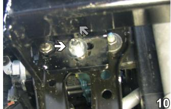
10. Hold the baseplate up in place and start the 8MM-1.25 x 50MM hex bolt (white arrow) with lock and two flat washers into existing hole, make it snug. Using the baseplate as a template, drill the hole above (gray arrow). Do this to both sides using a 13/32" drill bit.
