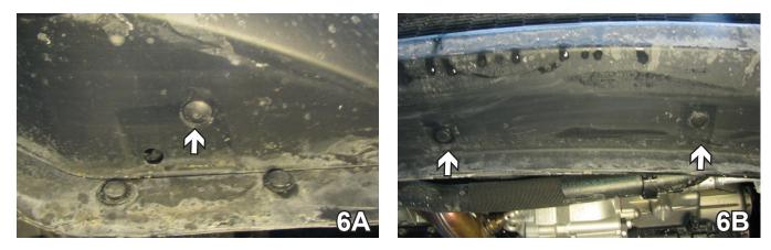
There is also a torx 25T bolt (photo 6A) to be removed from both sides using a torx wrench. Remove the three (3) push pins in the center (photo 6B). Pull the fascia forward, disconnect side running and fog lights. Set aside carefully for later reinstallation. Page 4 of 7 405-0048 Rev. C 9/24/19
