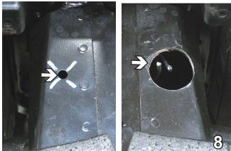
Using an existing hole on top of the metal bumper drill a hole using a 1 1/4" hole saw to cut opening for front end to install nut plates. Do this on both sides.
