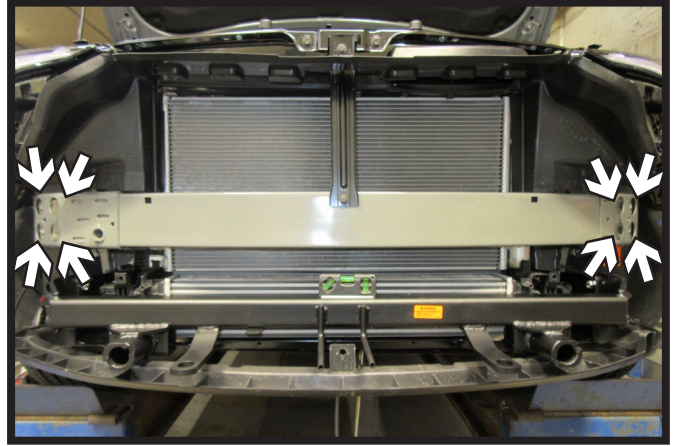
13. Install baseplate onto vehicle between frame and bumper. Level and reinstall the eight (8) existing 10MM bolts.
