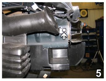
5. Remove pushpin from the passenger's side air baffle. Set air baffle and pushpin aside to reinstall later.
