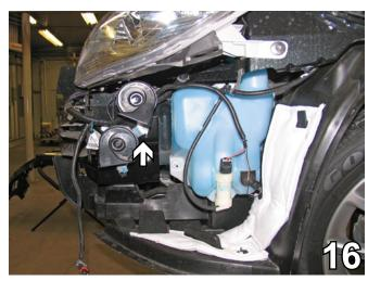
16. Reinstall the horn on the driver's side.
