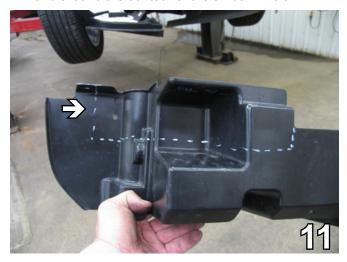
11. Also on the driver's side, mark straight down from the air dam tab three inches and horizontally back to the air dam contour and trim this area with the utility knife.
