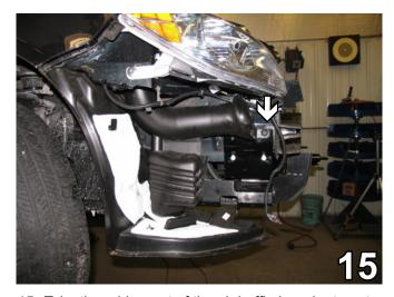
15. Take the rubber out of the air baffle in order to get the plug back in it.
