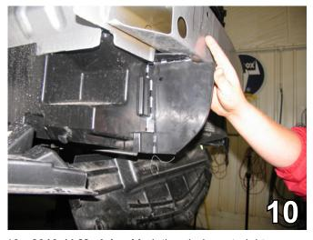
10. **2010-11 Models:** Mark the air dam straight across the top and straight down the side, as shown, and trim.
