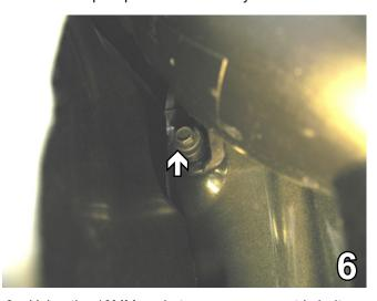
6. Using the 10MM socket, remove one metric bolt from the back side of the air baffle. Set air baffle and bolt aside to reinstall later.
