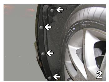
Just forward of the front tire, on the edge of the wheel well cover, remove four pushpins. Do this to both sides of the vehicle. Set pushpins aside to reinstall later.
