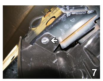
7. Remove pushpin from the bottom of the bumper. Do this on both sides. Set pushpin aside to reinstall later.
