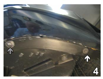
4. Using the 7MM socket, remove nine metric bolts from underneath corner of the front fascia, forward of the front tire, as indicated by the white arrow in the photo above. Remove two pushpins, as indicated by the grey arrow in the photo above. Do this around the vehicle. Remove fascia by pulling it out to the side and forward a little bit. Set fascia, bolts and pushpins aside carefully to reinstall later.
