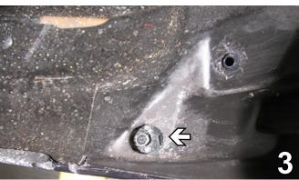
Also just forward of the front tire, on the edge of the wheel well cover, using the 10MM socket, remove the bolt. Do this to both sides of the vehicle. Set bolts aside to reinstall later.
