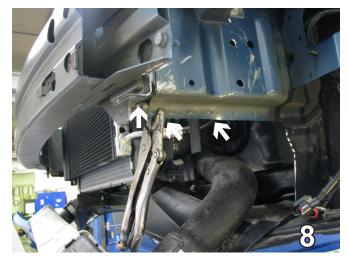
8. Using a vise grip, bend up where we just cut and continue to bend back to the middle of the rib. This is done on both sides of the vehicle.
