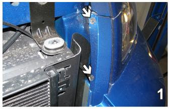
1. Using the 7MM socket remove two 7MM bolts from the front fascia near the headlight housing. This will need to be done to both sides of the vehicle, the driver's side is shown. Set bolts aside to be reinstalled later.
