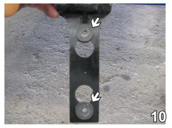
10. Remove the two grommets from each bracket, they will be used with the new bracket.
