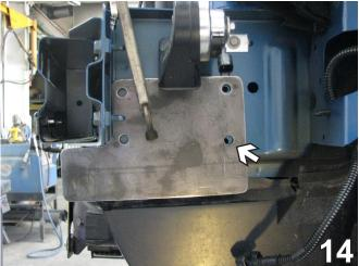
14. Align the baseplate with the existing hole. Clamp across the top of the frame with the large vise grip. This is done on both sides of the vehicle.
