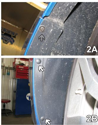
2. Just forward of the front tire, remove one 7MM bolt with the 7MM socket (see grey arrow) and remove two push pins (see white arrows). This is done on both sides of the vehicle, the driver's side is shown. Set all aside to be reinstalled later.
