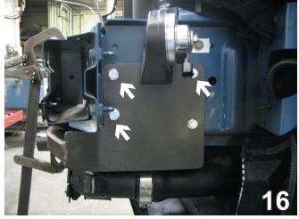
Insert three more 3/8-16 x 1 1/4" hex bolts with 3/8" lock washers and attach to 3/8-16 nut plates. Be sure to use Loctite. This is done on both sides of the vehicle.
