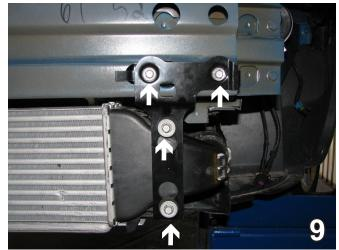
This bracket needs to be replaced. Using a 10MM socket, remove the four bolts holding the bracket. This is done on both sides of the vehicle. Set the bolts aside to be used later in reinstalling the new bracket.
