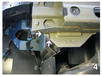
4. Underneath the bumper cut a notch across the bottom and flush with the side. This will need to be done on both sides of the vehicle, the passenger's side is shown.
