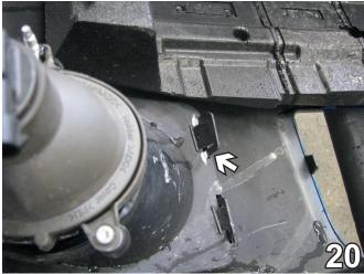
20. On the back side of the fascia, use a utility knife to cut the tall tab off. This is done on both sides of the vehicle. Reinstall the front fascia.
