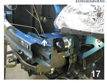
17. Cut the excess wire from the nut plates once they are installed. This is done on both sides of the vehicle.
