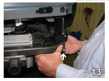
13. Continue to move the baseplate and the turbo on up into position. This is done on both sides of the vehicle.
