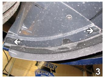
3. Just forward of the front tires, on the under side of the front fascia, remove two push pins. This is done on both sides of the vehicle, the driver's side is shown. Set the push pins aside to be reinstalled later. Pull fascia forward and set aside carefully to be reinstalled later.
