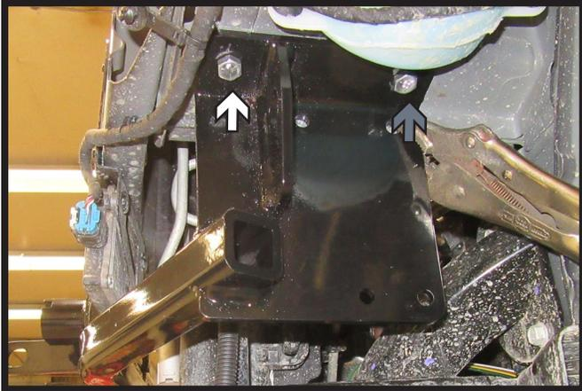
7. Slide the baseplate on and clamp into place. Install the provided 3/8" hardware into the existing holes on both sides of the vehicle (white). Using a 3/8" drill bit, drill out the back holes (gray) and install the 3/8" hardware.
