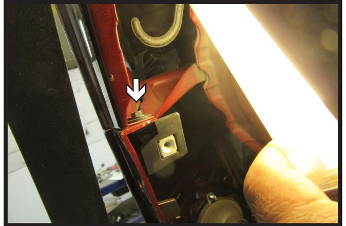
4. Pull the wheel well cover aside. Using a 7MM socket, remove the one (1) bolt from inside the fascia.
