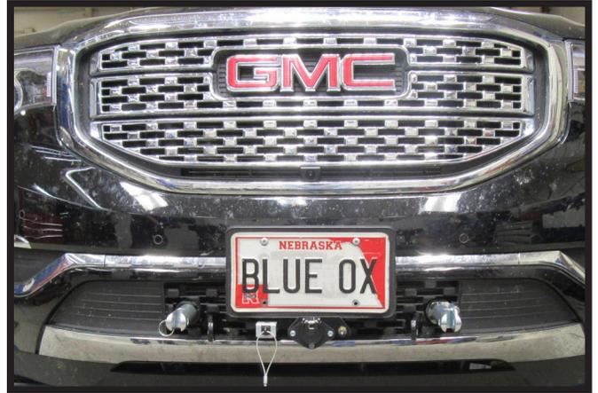
12. Hold the fascia as close to its original position, mark and trim the fascia around the convenience links and attachment tabs. Reinstall the fascia and fascia cover.
