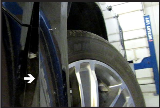
3. Carefully remove the plastic panel from the both sides of the vehicle.
