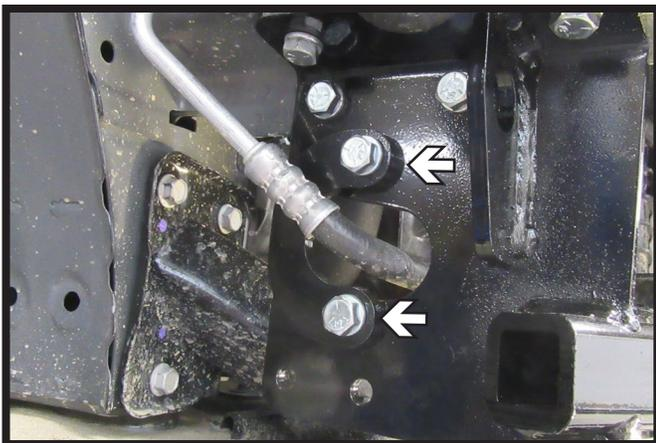
9. On the passenger side, attach the reinforcement brace around the line. Install with the provided 3/8" hardware.
