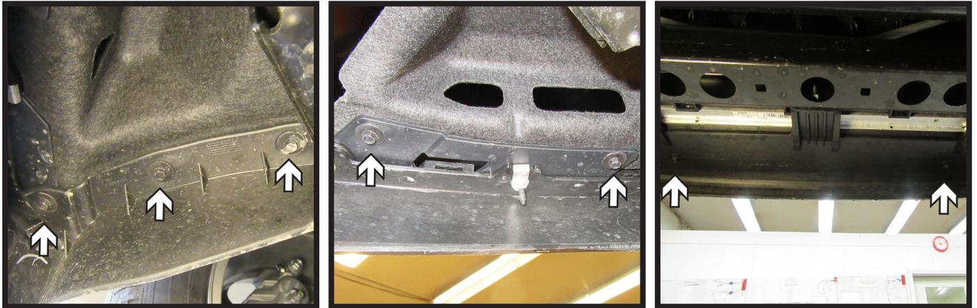
5. Using a 7MM socket, remove the ten (10) bolts from the underside of the car. There are three (3) in front of each tire, two (2) on each side of center, and two (2) in the center.
