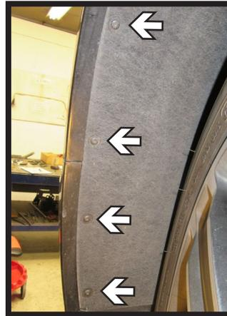
2. Using a T15 Torx, remove the four (4) screws from the wheel well in front of the tire. Do this for both sides of the vehicle.
