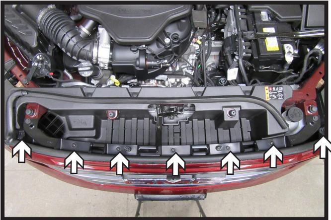
1. Using a T15 Torx, remove the seven (7) screws from the top edge of the fascia.
