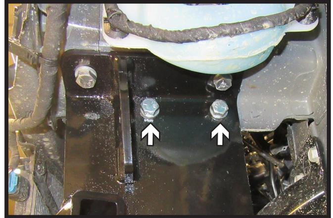
8. Using a 3/8" drill bit, drill out the holes on both sides of the baseplate, and insert the provided 3/8" hardware.
