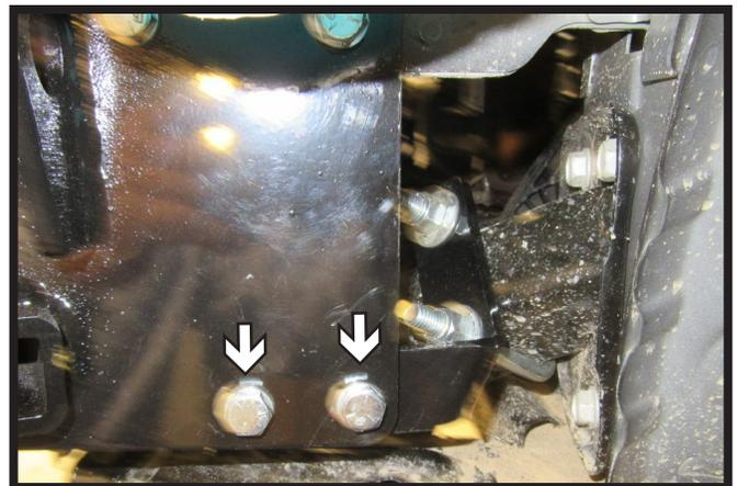
10. Secure U-bolt around the frame extension behind the baseplate, and install to baseplate with the provided brace and associated 3/8" hardware.
