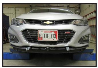
13. Hold the fascia as close to its original position, mark and trim the fascia around the convenience links and attachment tabs. Reinstall the center brace, headlights, fascia and fascia cover.
