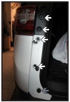
Unpop the covers for the five (5) bolts on the back panel of the vehicle. Then using a 7MM socket, remove the four (4) top bolts (white) and a T20 Torx to remove the one (1) bottom bolt (gray). Do this on both sides of the vehicle.
