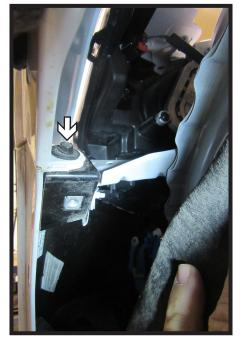
4. Pull back the wheel well liner. Using a 7MM socket, remove the one (1) bolt at the fascia joint. Do this on both sides of the vehicle.
