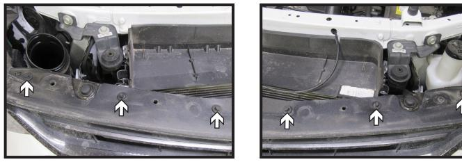
2. Using a 7MM socket, remove the six (6) bolts, three (3) on each side, from the top of the fascia.
