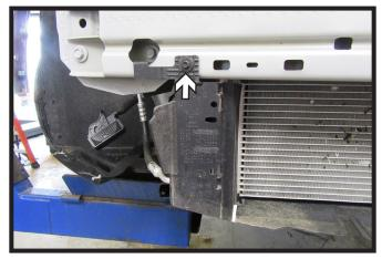
Using a 7MM socket, remove the two (2) bolts, one (1) on each side from the shutter housing. Using a utility knife remove the side pieces of the shutter housing as indicated.
