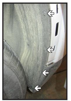
3. Using a T15 Torx, remove the four (4) bolts from the wheel well behind the rear tire. Do this on both sides of the vehicle.
