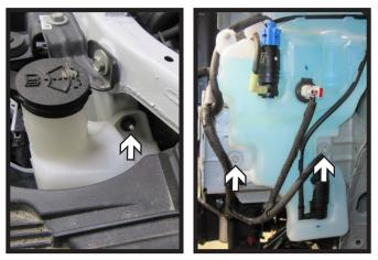
On the driver side of the vehicle, using a 10MM socket, remove the one (1) nut from the top of the windshield washer fluid reservoir. Disconnect all lines. Then using a 10MM socket, remove the two (2) bolts at the bottom of the reservoir.
