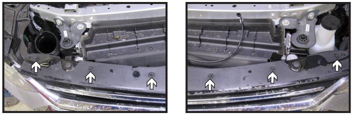
2. Using a 7MM socket, remove the six (6) bolts, three (3) on each side, from the top of the fascia.
