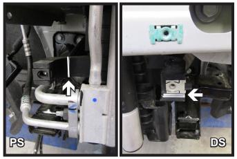
Using a reciprocating saw, trim the brackets on the driver and passenger sides of the vehicle as indicated to allow clearance for the baseplate.
