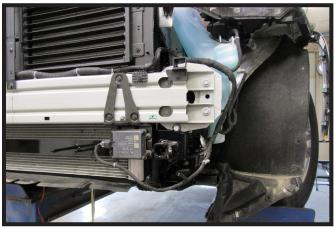
Reinstall the ACC and the windshield washer fluid reservoir on the driver side of the vehicle.
