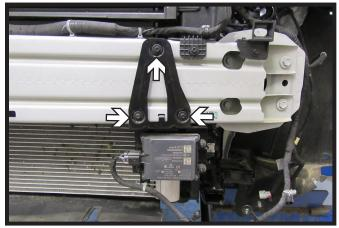
10. Using a 7MM socket, remove the three (3) bolts from the ACC bracket on the driver side of the vehicle. Remove bracket and set aside to be reinstalled later.
