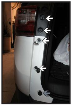
Unpop the covers for the five (5) bolts on the back panel of the vehicle. Then using a 7MM socket, remove the four (4) top bolts (white) and a T20 Torx socket to remove the one (1) bottom bolt (gray). Do this on both sides of the vehicle.
