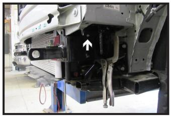
Using a 3/8" drill bit, drill the top front hole. Install 3/8" hardware. Do this on both sides of the vehicle. Remove vise grips.
