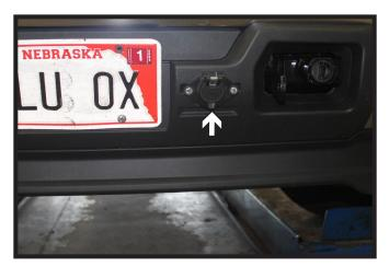
20. **Optional Silverado/Sierra Models:**Prior to fully reinstalling the fascia. Drill a hole thru the bumper at the desired location to accommodate the plug and bolts. Using 1/4" x 1-1/2" bolts with 1/4" washers, install the plug thru the bumper. On the backside of the bumper, install the electrical bracket and 1/4" locknuts to secure the plug to the bumper.
