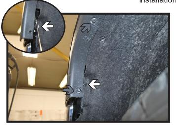
3b. **Sierra 1500 Models:** Using a 7MM socket, remove the screw from the wheel well (white). Using a T15 Torx, remove the screws (gray).
