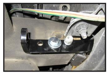
15. **All Models:** Remove the front bolt and then line up the convenience link on the inside of the frame. Insert both 1/2" bolts in opposite directions with washer and nylon lock nut and tighten fully. Tighten the bottom bolt at this time. Do this for both sides of the vehicle.
