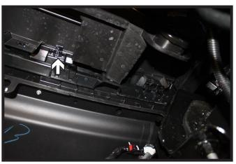
7b. Sierra 1500 Models: Unsnap the six(6) tabs from the backside of the fascia.Remove the fascia from the vehicle and set aside.
