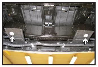
6. **All Tahoe/Suburban Models:** Using a 10MM socket, remove the two (2) remaining screws from the underside of the fascia.
