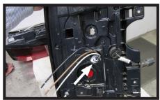
Drill a hole according to the tail light wiring kit instructions.
