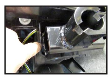
13. **All Models:** Slide the baseplate into place. If the baseplate does not slide in, tap the edges of the housing outward slightly. Do this on both sides of the vehicle.
