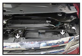
2b. **All Silverado/Sierra Models:** Using a 10MM socket, remove the four (4) screws from the top edge of the grille. There are two (2) on each side.
