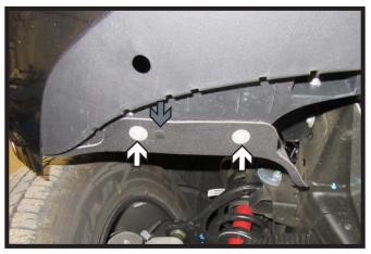
4. **All Tahoe/Suburban Models:** Using a 10MM socket, remove the six (6) screws from the underside of the fascia. There are three (3) on each side. Remove the two (2) push pins located in front of the tires (gray).
