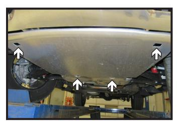
All Z71 Models: Using a 16 MM socket remove the four (4) bolts, two (2) in the front and back, attaching the belly pan.
