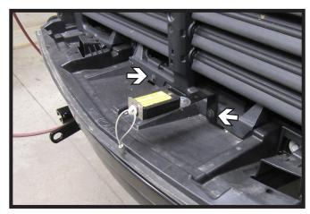
19. Optional Tahoe/Suburban Models: Using either existing bolt attach the brakeaway bracket. Then use a 1/4" bolt to attach the brakeaway switch to the bracket.
