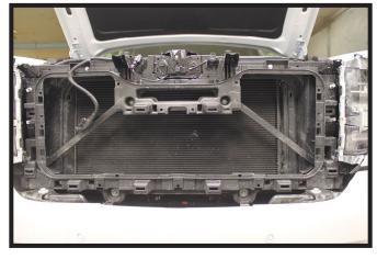
8. **All Sierra 1500 Models:** Using a 10MM socket, remove the four (4) screws from the bottom edge of the grille. There are two (2) on each side and set the grill aside (left).
