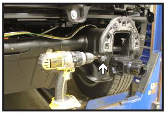
14. **All Models:** Insert the front 1/2" bolt and start the bottom 1/2" bolt with slotted plate and 1/4" thick washer, do this on both sides of the vehicle. Do not fully tighten the bolts. **Note:** The bottom frame hole may need to be reamed out to align with the slot.
