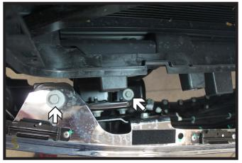
All Silverado/Sierra Models: Using a 18MM socket, remove the four (4) bolts from the top of the bumper. There are two (2) on each side. Set the bumper aside.
