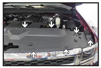
All Models: Remove the twelve (12) push pins from the shroud cover. There are six (6) on each side. Set the cover aside.
