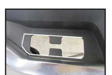
17a. **All Tahoe/Suburban Models:** On the inside of the fascia trim the indicated area to allow the attachment tabs and convenience links to fit through. Do this on both sides of the fascia.
