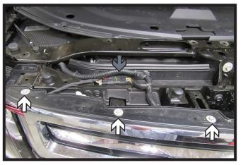
2a. **All Tahoe/Suburban Models:** Using a 10MM socket, remove the six (6) screws from the top edge of the fascia (white). There are three (3) on each side. On the passenger side, disconnect the wiring harness (gray).
