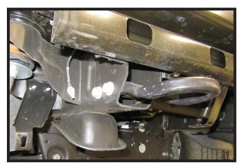
12a. **All Tahoe/Suburban Models:** Using a 18MM socket remove the six (6) bolts, three (3) on each side, attaching the tow hooks and remove tow hooks. Do this on both sides of the vehicle.
