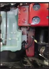
6. Remove the push pin (white) from the top of the windshield washer fluid reservoir on the passenger side of the vehicle. Then using a 10MM socket, remove the two (2) nuts (gray) and one (1) bolt (black) from the reservoir. Plug all lines, remove reservoir, and set aside to be reinstalled later.
