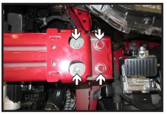
Using a 15MM socket, remove the four (4) bolts from the front of the bumper. Do this on both sides of the vehicle. Let bumper hang.
