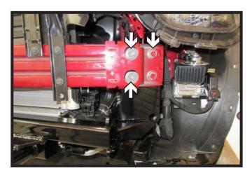
13. Install the remaining three (3) existing 10MM bolts on each side of the vehicle. Then remove starter bolt from each side and apply Locitie® Red and reinstall.
