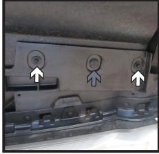
5. Using a 7MM socket, remove the six (6) bolts (white) from the underside of the fascia. Then remove the two (2) push pins (gray). Unplug electrical connections and remove fascia. Set fascia aside to be reinstalled later.
