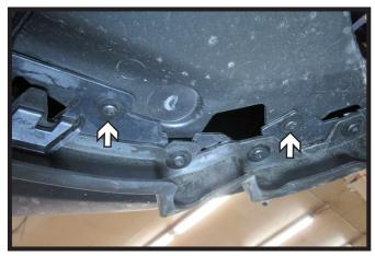
4. Using a T15 Torx, remove the four (4) bolts from the underside of the fascia in front of the tire. There are two (2) bolts on each side of the vehicle.
