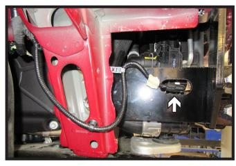
Reconnect electrical on passenger side of the vehicle through the hole in the support plate.
