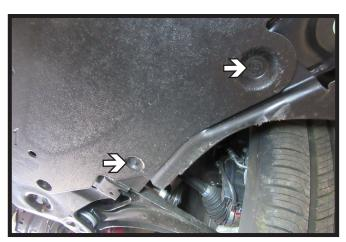
10. Using a 7MM socket, remove the front two(2) bolts on each side of the belly pan. Let belly pan hang.
