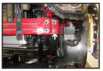
12. Slide the baseplate between the bumper and the frame. Start one (1) existing bolt on each side of the vehicle to hold baseplate in place.
