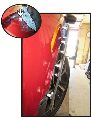
3. Pull back the wheel well trim and prop away from the vehicle using a soft cloth. Then using a 7MM socket remove the one (1) bolt from the fascia joint (inset). Do this on both sides of the vehicle.
