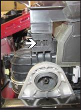
7. Remove the shroud below the bumper by cutting the indicated area. Then press clip on bottom of shroud to slide forward and off of the vehicle. Do this on both sides of the vehicle.
