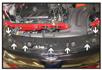
Using a T15 Torx, remove the seven (7) bolts from the top edge of the fascia.
