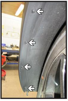
Using a T15 Torx, remove the four (4) bolts from along the edge of the wheel well. Do this on both sides of the vehicle.
