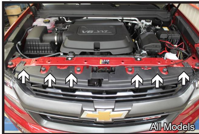
1. **Canyon Only:** Remove the nine (9) push pins, four (4) on each side and one (1) in the center, from the fascia cover. Set aside cover to be reinstalled later.
