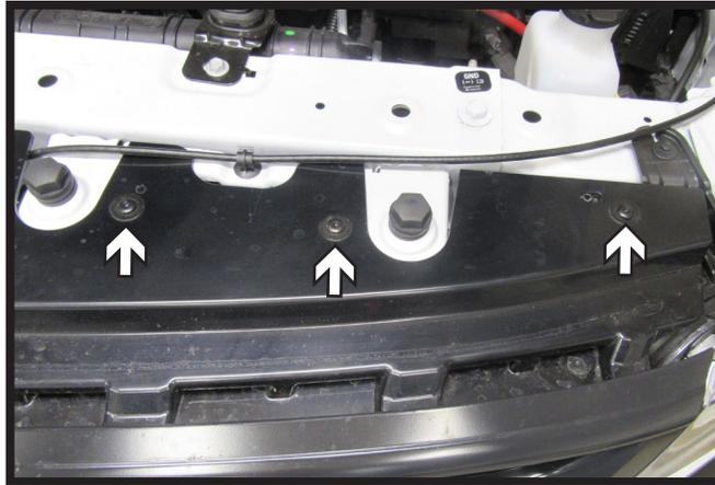
1. Using a T15 Torx, remove the six (6) screws, three (3) on each side, from the top edge of the fascia.
