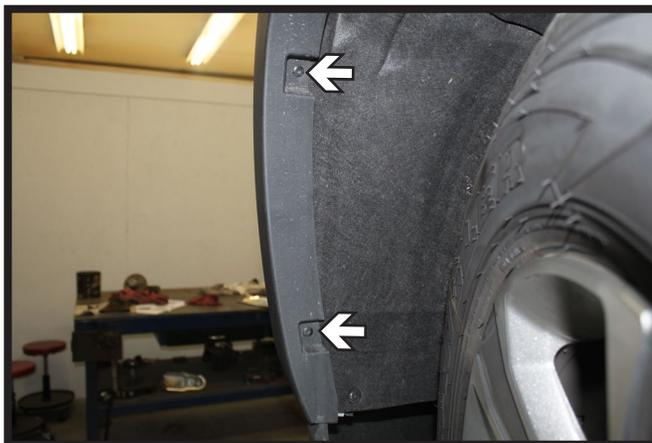
2. Using a T15 Torx, remove the four (4) screws from the edge of the fender flare. Do this on both sides of the vehicle.
