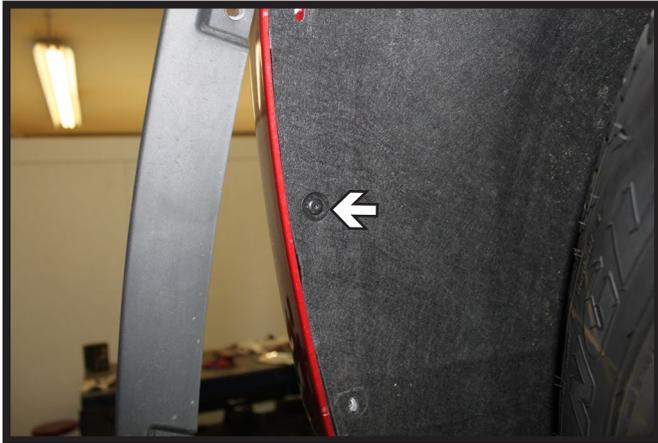
3. Pull out the fender flare and remove the screw behind, using a T15 Torx. Do this on both sides of the vehicle.
