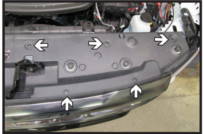
1. Remove the nine (9) push pins from the fascia cover. Remove fascia cover and set aside to be reinstalled later.
