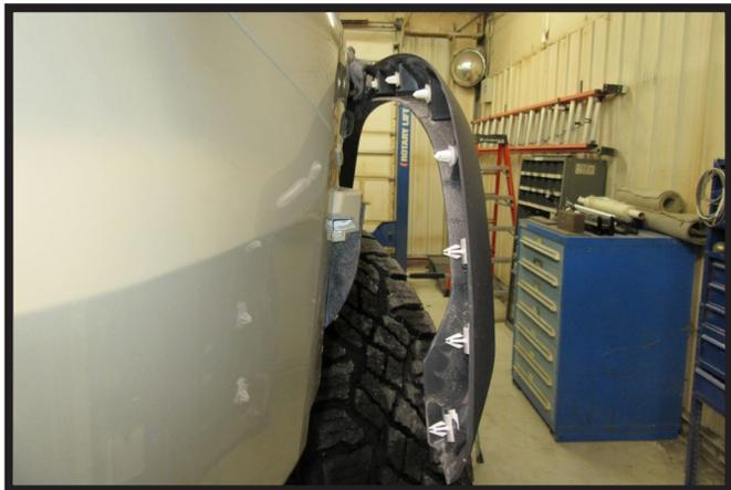
4. Unclip the wheel well trim and prop away from the vehicle using a soft cloth. Do this on both sides of the vehicle.
