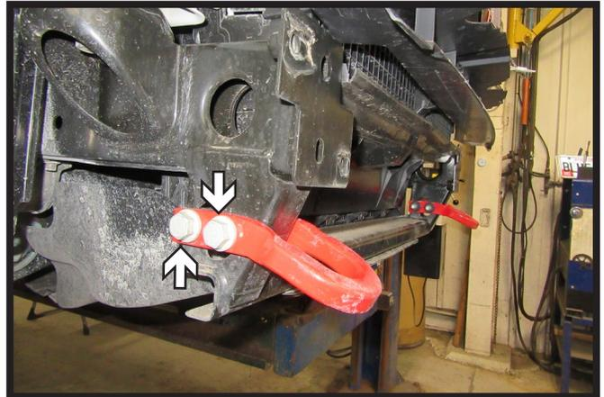
2. Using an 18MM socket and wrench, remove the two (2) bolts from the tow hook. Do this on both sides of the vehicle. Remove the tow hooks and set aside. They will not be reinstalled later.
