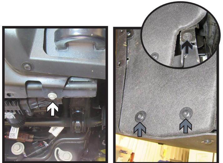
6. Using a 10MM socket, remove the one (1) screw (white) from under the tow hook. Then using a T15 Torx remove the two (2) indicated screws (gray). Using a 7MM socket remove the one (1) screw as indicated in the inset (black). Do this on both sides of the vehicle.
