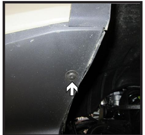
3. Using a T15 Torx, remove the six (6) bolts from along the edge of the wheel well and under the vehicle. Do this on both sides of the vehicle.
