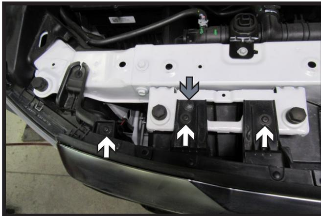
2. Using a T15 Torx, remove the six (6) bolts (white) and two (2) push pins (gray) from the top edge of the fascia. There are three (3) bolts and one (1) push pin on each side.
