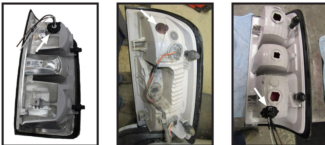
Drill a hole according to the tail light wiring kit instructions.
