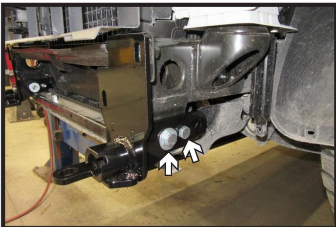
3. Slide baseplate into place and insert two (2) 1/2" x 3-1/2" bolts into the side holes. Use a flat washer with front bolt. Do not install nuts at this time. Do this on both sides of the vehicle.
