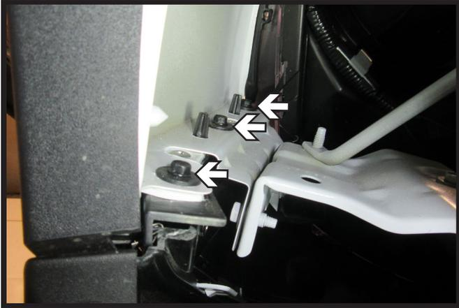
3. Behind the wheel well liner, using a 7MM socket, remove the three (3) screws along the fascia/fender joint. Do this on both sides of the vehicle.
