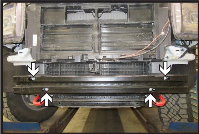
1. Using a 15MM socket, remove the four (4) bolts from the bumper. There are two (2) bolts on each side of the vehicle. Remove bumper and set aside to be reinstalled later.
