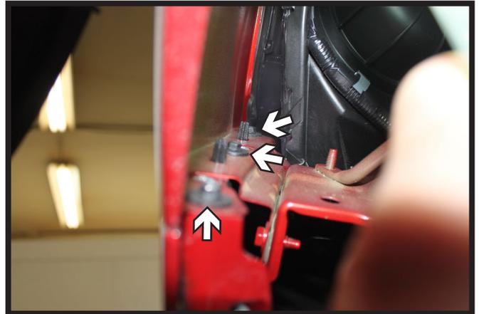
4. Behind the wheel well liner, using a 7MM socket, remove the three (3) screws along the fascia/fender joint. Do this on both sides of the vehicle.
