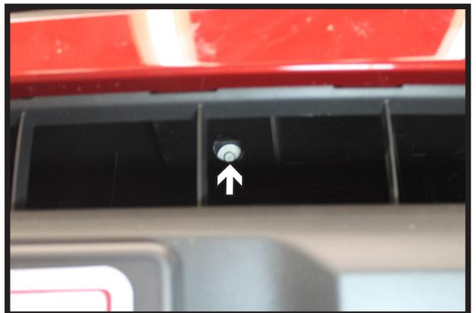
6. Using a 10MM socket, remove the two (2) screws from inside the grill just above the license plate bracket. There is one (1) on each side.
