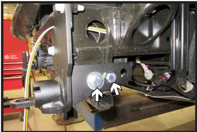
5. Remove the two (2) side bolts, add Loctite Red, and reinstall. Tighten fully at this time. Do this on both sides of the vehicle.
