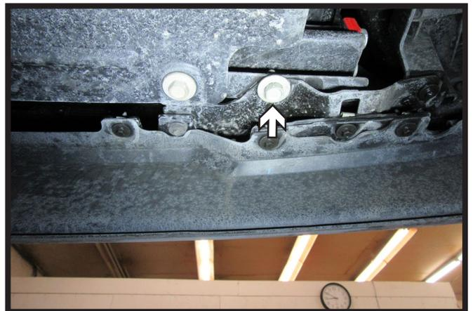
7. Using a 15MM socket, remove the one (1) bolt from the underside of the fascia. Do this on both sides of the vehicle. Remove fascia and set aside to be reinstalled later.
