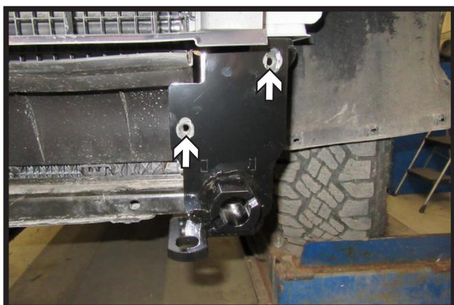
7. Remove the two (2) bolts from the front of each baseplate (left). Reinstall the bumper, then reinstall the existing bolts using Loctite Red (right). Tighten fully at this time.
