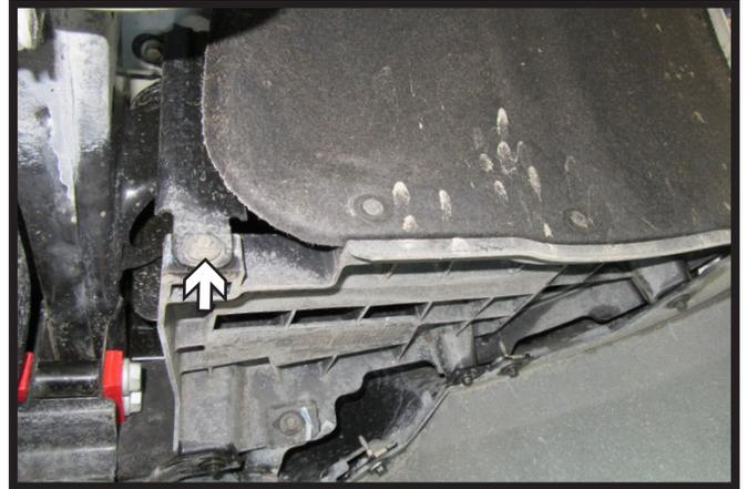
5. Using a 7MM socket, remove the one (1) bolt in front of the tire. Do this on both sides of the vehicle.
