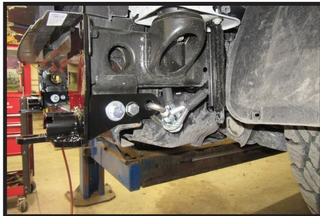
6. Before reinstalling bumper, attach the permanent baseplate safety cables to the provided convenience link on the baseplate. The photo above shows the recommended installation of the cables to frame of vehicle. Additional options may interfere with suggested mounting; in this case, secure the cables to a solid piece of the frame as described in the General Information sheet. Be sure the safety cables do not rub against any hoses or moving parts. Do this on **BOTH** sides of the vehicle.
