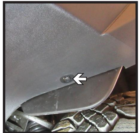
2. Using a T15 Torx, remove the five (5) screws from in front of the tire in the wheel well. Do this on both sides of the vehicle.
