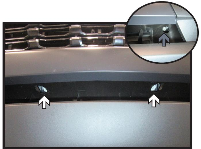
4. Using a 10MM socket, remove the two (2) screws (white) from the grill just above the license plate bracket.
