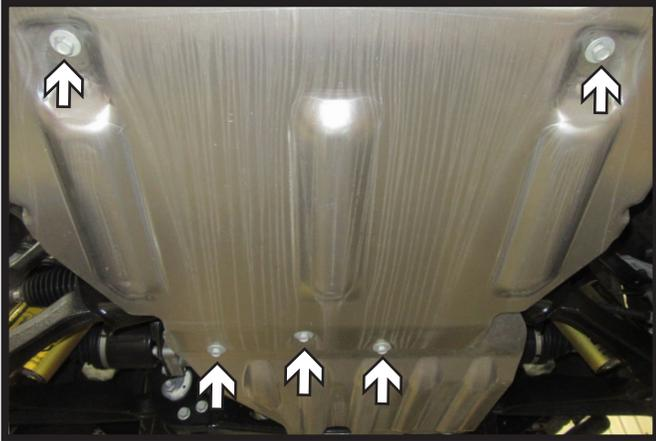
1. Using a 15MM socket, remove the five (5) bolts from the skid plate. There are two (2) bolts towards the front and three (3) towards the back. Remove skid plate and set aside to be reinstalled later.
