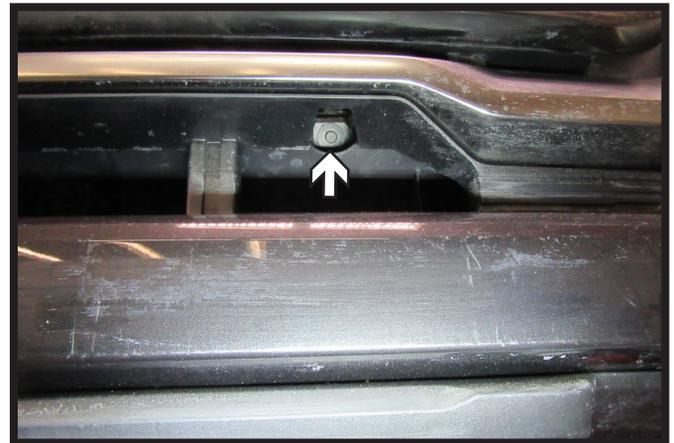
3. Using a 10MM socket, remove the two (2) bolts from the grille. There is one (1) bolt on each side of the vehicle.
