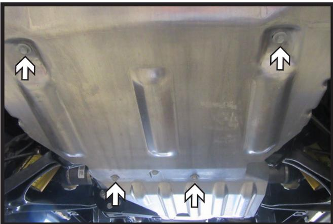
5. Using a 15MM socket, remove the four (4) screws from the belly pan. Remove belly pan and set aside to be reinstalled later.
