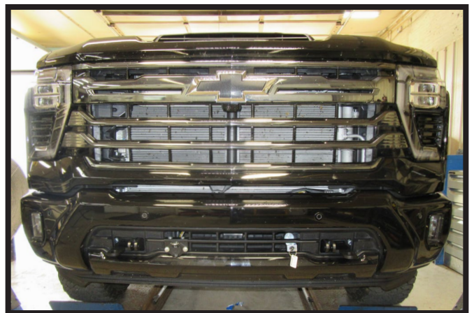
23. Reinstall bumper, grille, fascia, fascia cover and handle. Reconnect all electrical connections and hoses.
