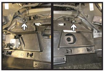
19. Unclip the wire loom on each side from the cover. Remove cover from the back of the fascia and set aside to be reinstalled later.
