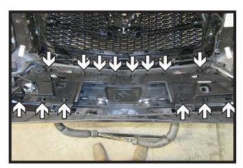
18. Unclip the fourteen clips, six (6) on the bottom and eight (8) on the top, from the cover on the back of the fascia.
