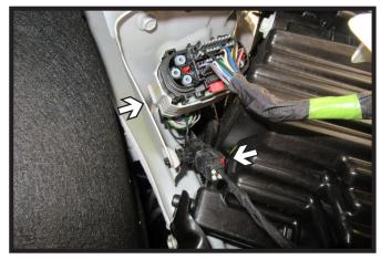
7. As the fascia is removed, unplug the two (2) electrical connections on the passenger side. Remove fascia and set aside to be reinstalled later.
