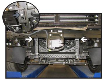
8. Using a reciprocating saw, cut the top of the plastic piece on each side as indicated. Then using a 10MM socket, remove the two (2) bolts, one (1) on each side, from the bottom of the plastic piece (inset). Remove plastic piece, it will not be reinstalled.
