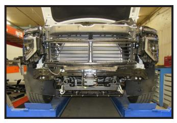
20. Reinstall plastic shroud above the bumper and reconnect wire loom.
