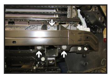
13. Using a 15MM socket, remove the six(6) bolts, three (3) on each side from the bumper. Remove bumper and set aside to be reinstalled later.
