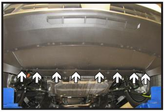
6. Using a 7MM socket, remove the eight (8) bolts from the bottom of the fascia.
