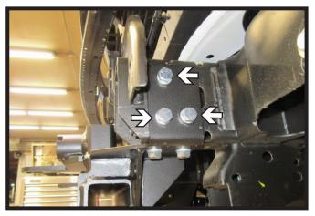
17. Insert three (3) 1/2" bolts with lock washers and whiz nuts. Do this on both sides of the vehicle.
