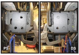
14. Slide the baseplate onto the vehicle and line up the holes of the baseplate as closely as possible to the existing holes in the frame. Clamp in place using large vise grips.
