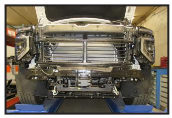
21. Reinstall bottom bolts and tighten upper nuts on top shutter housing.
