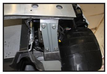
On the driver side, using a 14MM socket, remove the four (4) bolts from the bumper reinforcement bracket. The bracket will not be reinstalled.
