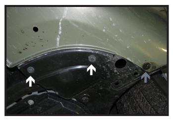
Using a 10MM socket, remove the two (2) screws from underside of the fascia (white). Then remove the outer push pin (gray). Do this on both sides of the vehicle.
