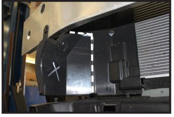
8. Trim the plastic shrouding just below the bumper back to the seam for baseplate clearance. Do this on both sides of the vehicle.
