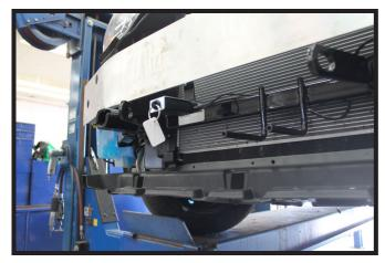
23. **Optional Breakaway:** Fasten the bracket to the underside of the bumper with a #10 screw at the desired location. Install the breakaway to the bracket with the supplied 1/4" bolt and lock nut.
