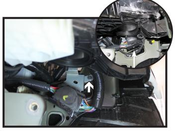
16. On the driver side, using a 10MM socket, remove the screw from the electrical bracket. Slide the bracket up the frame and reinstall in a higher position.
