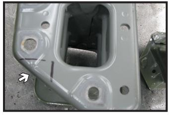
14. Temporarily reinstall the frame extensions and mark the backsides around the frame cuts. Remove the extensions and trim these areas with a reciprocating saw.
