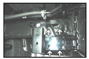
On the inner side of the frame, using the baseplate as a template, drill the two (2) upper frame holes and the two (2) bottom side frame holes with a 17/32" drill bit (white). Using a 1-1/4" hole saw, drill a hole in the frame above the bracket for access of the 1/2" nut wires (gray). Repeat on the other side of the vehicle.
