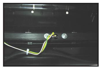
16. Attach the electrical connector with 5/16 x 3" bolts to 2" tubes, 5/16" flat washers and 5/16" nuts on the back side of the plastic insert.
