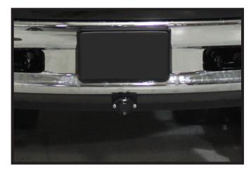
17. 2013 Models: Locate the electrical bracket to the desired location and mark the location of the bumper. Drill out attachment holes with a 1/4" drill bit. Install the bracket onto the bumper with 1/4" x 3/4" bolts and 1/4" lock nuts. Reinstall the air dam, mark for the electrical connector, then using the 1-1/4" hole saw drill a hole thru the air dam. Fasten the electrical connector to the bracket with 1/4" hardware.
