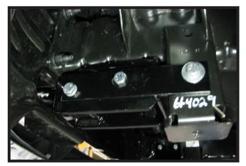
On the outer frame bolts, install 1/2" lock washers onto the front two (2) bolts. Then a 1/2" flat washer onto the rear hole. Fully tighten all bolts. Repeat on the other side of the vehicle.
