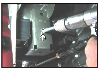
On the outer side of the frame, using a 17/32" drill bit, ream out the existing lower slot. Repeat on the other side of the vehicle.
