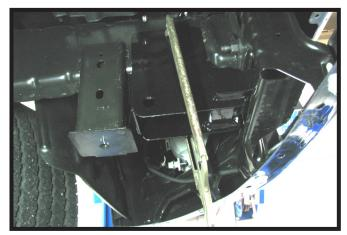
5. Tip the baseplate at an angle, then slide it into the opening and up to the frame. Clamp the baseplate to the frame.
