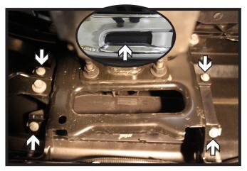
2013 Models without Tow Hooks: Using a 10MM socket, remove the four (4) screws from the bumper cover and slide out. Repeat on the other side of the vehicle. These covers will not be reinstalled.
