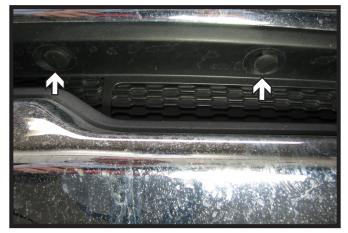
1. **2009-12 Models:** Remove the six (6) push pins along the front plastic insert and remove from the vehicle.
