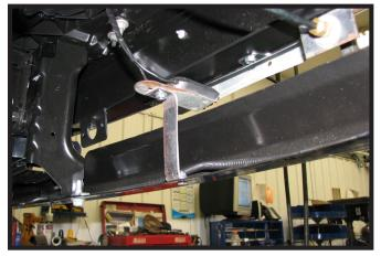
Reinstall the lower plastic bumper. There are three holes in the plastic where the breakaway bracket can be attached using a 1/4-20 x 3/4" bolt with a 1/4-20 nut. Attach the breakaway to the top of the bracket also with a 1/4-20 x 3/4" bolt and a 1/4-20 nut.
