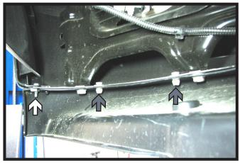
To remove the lower air dam, use a 10MM socket and remove the two (2) bolts in each corner of the air dam (white). Remove the thirteen (13) push pins along the seam (gray).
