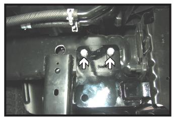
On the upper frame holes, insert 1/2"-13 x 1-1/2" bolts with 1/2" lock washers and 1/2" nut wires and tighten down. Repeat on the other side of the vehicle.
