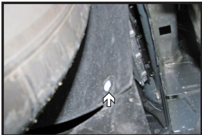
4. On the driver side only, remove the push pin in the inner wheel well.
