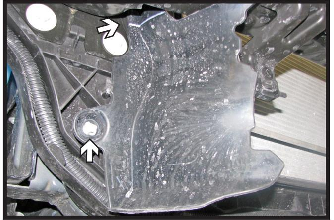
7. Trim the upper section of the shielding and remove the lower push pin. Do this on both sides of the vehicle.
