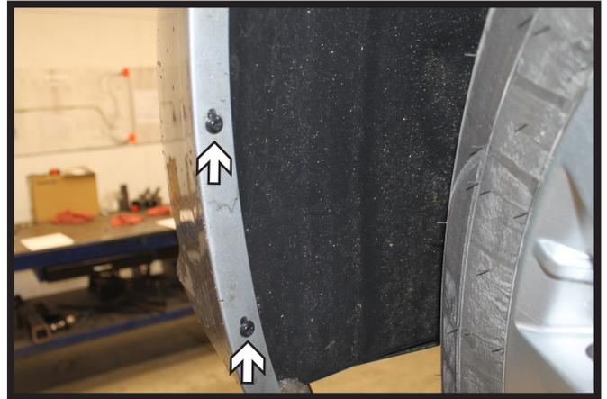
2. Using a Phillips screwdriver, remove the two (2) screws from along the edge of the wheel well. Do this on both sides of the vehicle.
