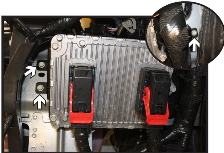
9. On the driver side, using a 10MM socket, remove the three (3) screws from ECM and set aside.
