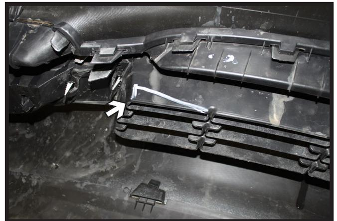
17. On the backside of the fascia, trim the corner as shown for baseplate clearance. Do this on both sides of the fascia.
