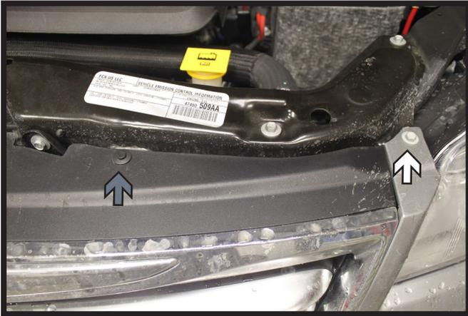
1. Using a 10MM socket, remove the screw from the top edge of the fascia (white). Then remove the push pin just to the inside of the screw (gray). Do this on both sides of the vehicle.
