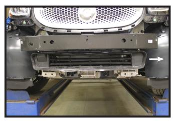
6. Slide the shroud towards the driver side and remove from the vehicle. The shroud will not be reinstalled.
