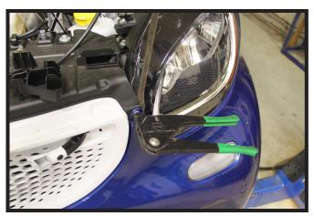
12. Once the fascia is reinstalled and any other installations are completed, pop rivet the fascia back to the vehicle using the provided plastic rivets.
