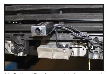
10. Optional Breakaway: Attach the bracket in the desired location flush with the outside of the aluminum tube with the 1/4" hardware. Install the breakaway to the bracket with the supplied 1/4" hardware.
