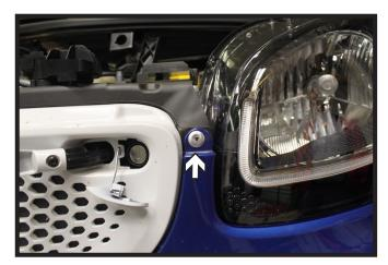
2. Using a 1/4" drill bit, drill out the rivet at the upper corner of the fascia by the headlight. Do this on both sides of the vehicle.
