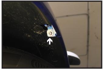
3. Using a T30 Torx, remove the screw from fascia/fender joint in the wheel well. Do this on both sides of the vehicle.
