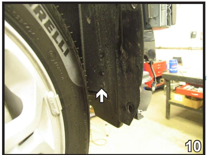
10. Using the 7MM socket, remove the screw from the wheel well. Set screw aside to be reinstalled later.
