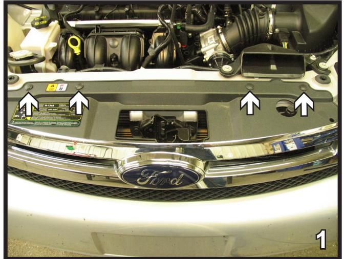
1. Remove four (4) Phillips push pins from radiator cover and lift to remove. Also remove grille assembly. Set push pins, radiator cover and grille aside to be reinstalled later.
