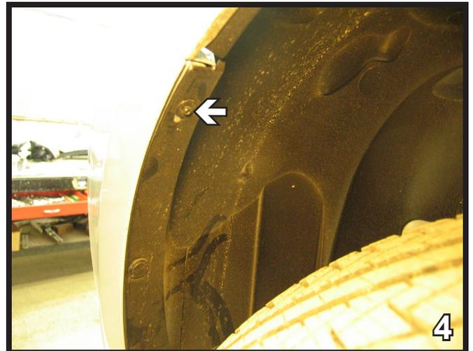
4. Using 6MM socket, remove one (1) screw from edge of fascia, just inside the wheel well. Do this to both sides of the vehicle. Set screws aside to be reinstalled later.
