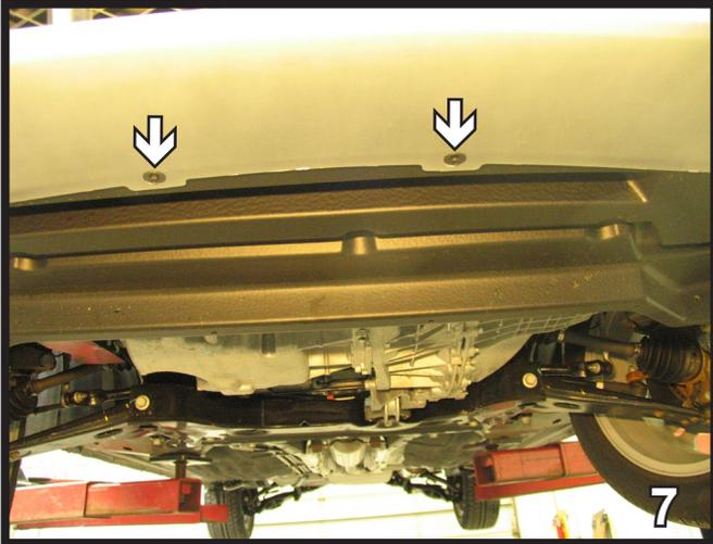
7. Using the 7MM socket, remove two (2) screws from the bottom center of fascia. Set screws aside to be reinstalled later. Pull fascia corner out to the side of vehicle, both sides, then pull fascia forward and set aside carefully for later reinstallation. Unplug the fog lights.
