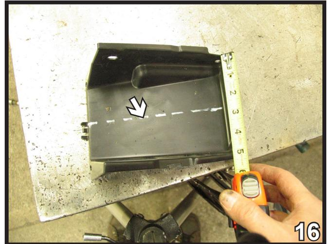
16. Trim the air dam, from the to edge take off 2-3/4". This allows clearance for the baseplate.
