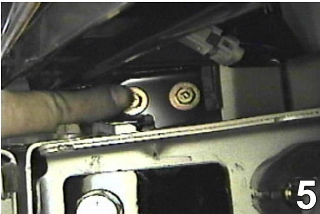
5. Using the 10MM socket, remove five bolts under and one on the outside of the headlight assemblies, unplug and set aside to be reinstalled later. Set metric bolts aside to be reinstalled later. Do this to both sides of the vehicle.
