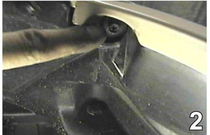
2. Using the 8MM socket, just behind the fascia's upper corner, remove one metric bolt. Set the bolt aside to be reinstalled later. Do this to both sides of the vehicle.
