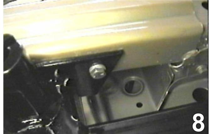
8. Reinstall the metal bumper, align the 3/8-16 nutplate inside the metal bumper with the drilled 13/32" hole and tighten the 1/2" lock washer, 3/8" lock washer. for upper supports.
