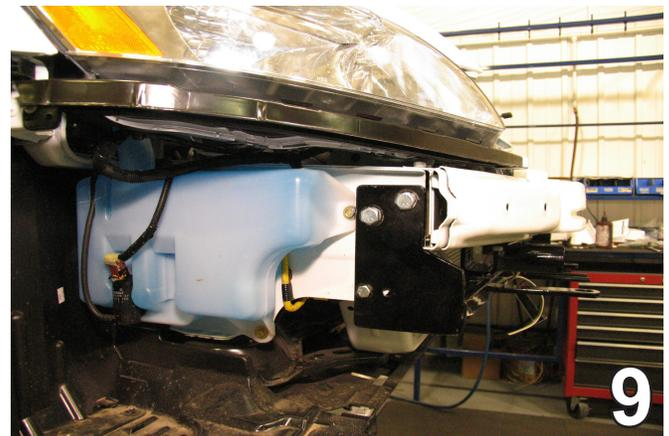
9. Reinstall the fascia and headlight assemblies. Some trimming may be required.
