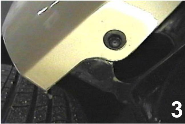
3. Using the 10MM socket, remove the metric bolt from the bottom side of the fascia corner. Set the metric bolt aside to be reinstalled later. Do this to both sides of the vehicle.
