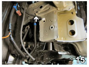
15. Relocate and secure the ground wire to the upper rear section of the frame rail on the passenger's side.
