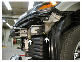
7. On the driver's side, use a 10MM socket to remove two metric bolts securing the air baffle. Pull down to remove. Set bolts and air baffle aside to be reinstalled later.
