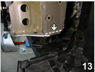
Using a reciprocating saw, cut the lip found at the bottom of the radiator support (dotted lines in graphic) to gain access to the area beneath it. Do this to both sides of the vehicle.
