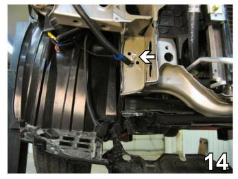
14. Using a 10MM socket, remove a ground wire from the forward facing section of the radiator support on the passenger's side.
