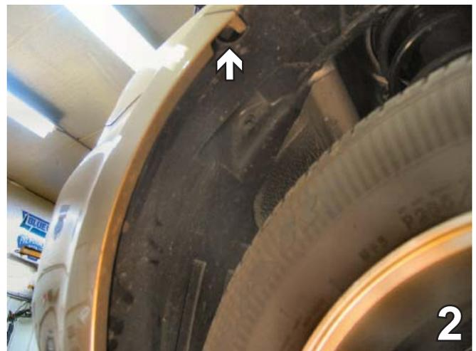
2. Above the front tire, inside the wheel well on the edge of the fascia, remove one Phillips screw. Do this to both sides of the vehicle. Set screws aside to reinstall later.
