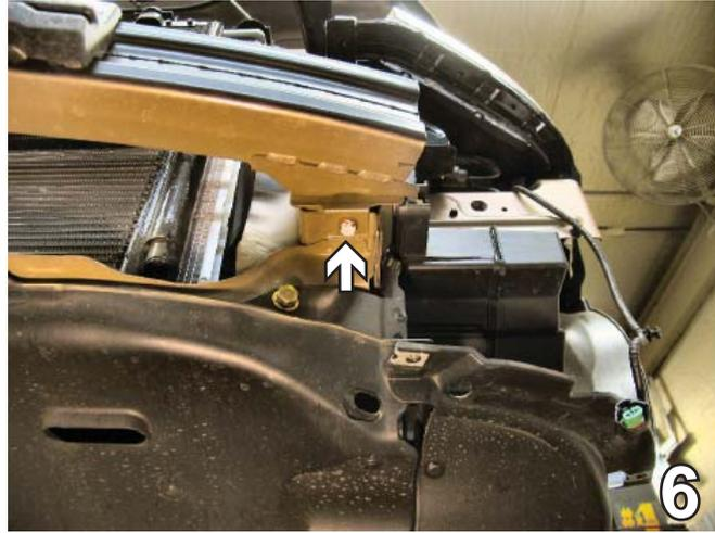
6. Using a 12mm socket, remove one metric bolt from the bottom of the metal bumper. Do this to both sides of the vehicle. Pull the bumper forward to remove. Set bolts and metal bumper aside to be reinstalled later.
