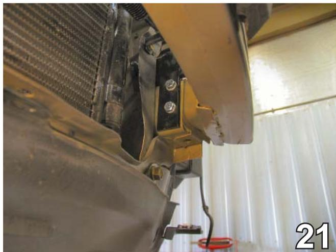
21. With the bumper off, insert 3/8-16 nutplate into the frame opening to align with drilled holes on the side of the frame rail. Insert the two 3/8-16 x 1 1/2" hex bolts and 3/8" lock washers and hand tighten. Metal bumper is only shown in photo for orientation
