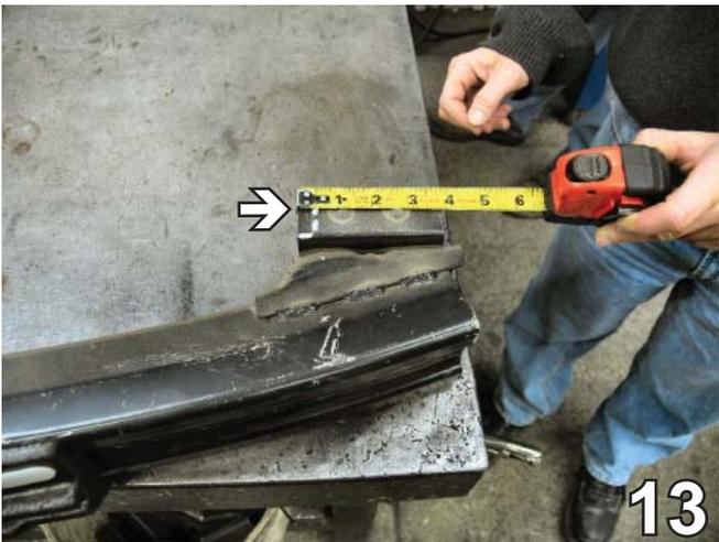
13. Mark and cut a section of the top bumper bracket edge that faces toward the center of bumper. Using the reciprocating saw, make a horizontal cut on the top of the bracket removing 3/8" from the end of the bracket. Do this to both sides of the bumper.
