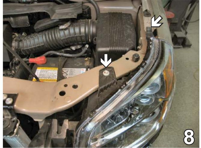
8. Using a 10MM socket, remove the metric bolt at the top of the headlight assembly. Remove the pushpin on top of the headlight assembly just above the front fender. Do this to both sides of the vehicle. Set bolts and pushpins aside to reinstall later.
