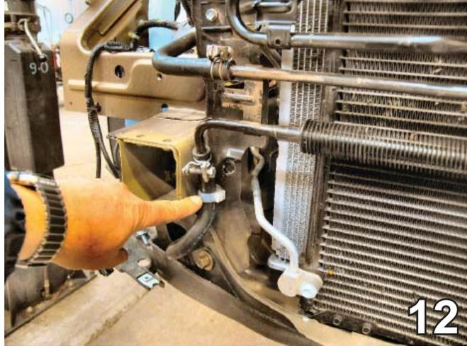
12. On the passenger's side, release the hose clamp found near the frame rail and slide the hose out of the clamp. Swivel the coolant line and hose to the left of the radiator support – moving the coolant line and hose away from the frame rail to clear that area for drilling.
