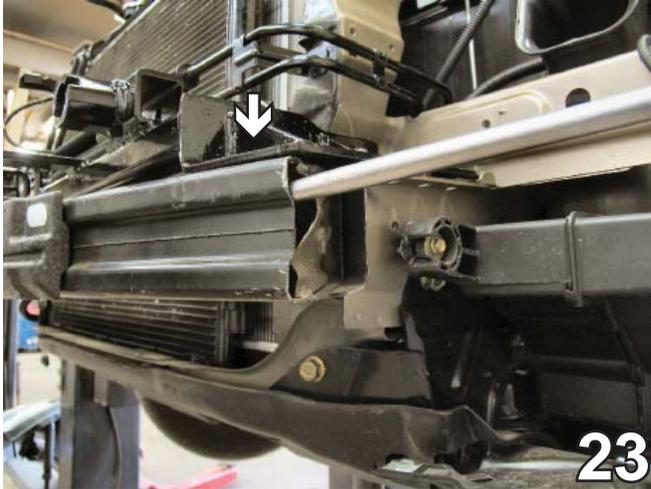
23. Put a pry bar or crow bar into the frame rail opening and create a larger opening for easier access to guide the nut plate through. Insert one 3/8-16 nut plate through the metal bumper opening and align with the hole in the top of the bumper and tighten to the hex bolt (see arrow). Do this to both sides of the vehicle. Arrow indicates hole that nutplate aligns with into bumper.
