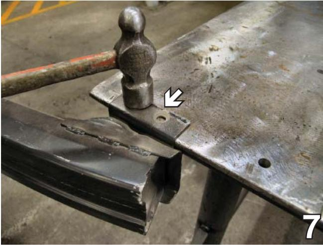
7. Lay the metal bumper's upper bracket on a solid metal surface. Pound the ridge on the bracket to flatten it and prepare it for baseplate installation. Do this to both sides of the metal bumper. Set bumper aside to reinstall later.
