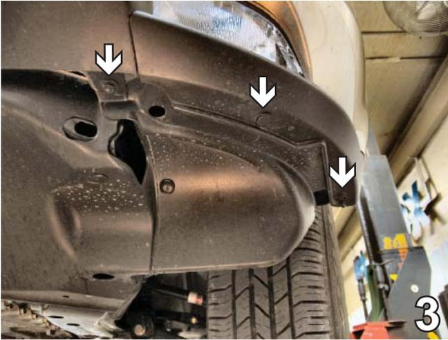
3. On the bottom edge of fascia, remove a pushpin and two metric bolts using a 10MM socket. Do this to both sides of the vehicle. Set pushpins and bolts aside to reinstall later.
