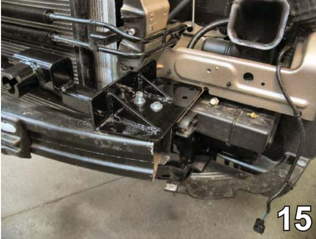
15. Slide the baseplate onto the top of the frame rail and guide the metal bumper between baseplate and the top of the frame rail. Align the two holes of the baseplate with the two holes on top of the metal bumper and frame. Insert two 8mm-1.25 x 30mm hex bolts and fasten (do not overtighten) with 8mm lock washer and 5/16" flat washer using a 13mm socket. Do **NOT** use Loctite yet.
