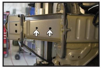
12. Using a 3/8" drill bit, drill out the two existing holes in the bumper. Do this on both sides of the vehicle.
