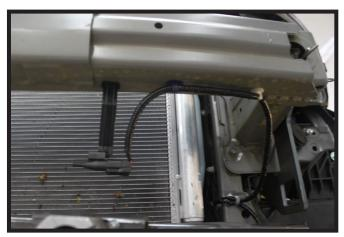
10. Remove the temperature sensor from the underside of the bumper and set aside.
