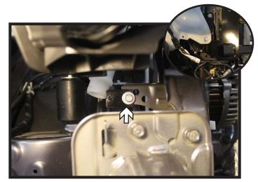
Install the washer reservoir bracket onto the upper existing hole with the existing screw. Reinstall the washer reservoir.
