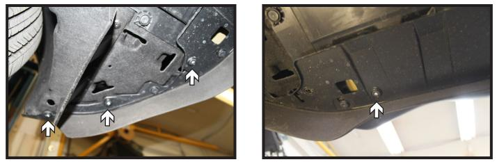
5. Remove the eight (8) push pins from the underside of the fascia. There are four (4) on each side.
