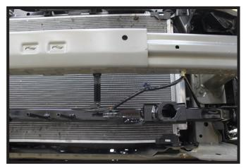
17. Using a 5/16" drill bit, drill a new hole for the temperature sensor on the underside of the bumper and reinstall the temperature sensor away from the attachment tube.
