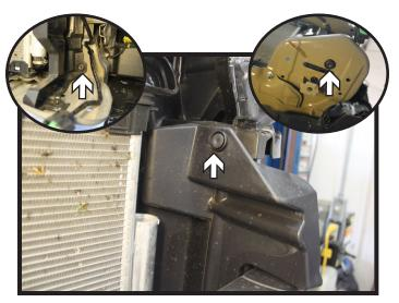
9. Remove the three (3) push pins from the plastic shielding and set aside. Do this on both sides of the vehicle. The shielding will not be reinstalled.
