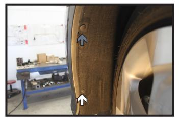
3. Using a phillips screwdriver, remove the screw from the lower edge of the wheel well (white). Then remove the push pins above the screw (gray). Do this on both sides of the vehicle.
