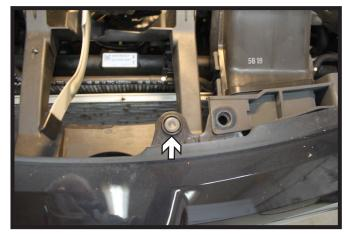
2. Remove the push pin from the top of the fascia.
