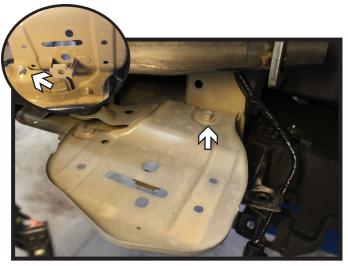
11. Using a 10MM socket, remove the bolt and nut from the metal shielding and set aside. Do this on both sides of the vehicle.
