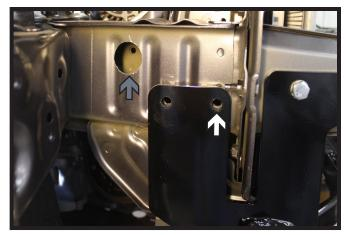
15. Using a 3/8" drill bit, drill out the two rear holes in the baseplate thru the frame. Do this on both sides of the vehicle.
