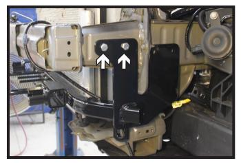
14. Position the baseplate onto the vehicle. Start the 3/8" hardware into the bumper holes on both sides of the vehicle and level the baseplate. Once the baseplate is level, fully tighten all hardware.
