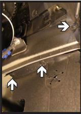
10. Using a 10MM socket, remove the three (3) screws from the washer reservoir. Then remove the one (1) push pin from the filler neck (left).
