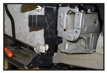
13. Trim the plastic shielding just above the frame pocket, then remove the lower push pins holding it in place. Do this on both sides of the vehicle.
