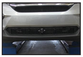
16. Hold the fascia as close to its original position, mark and trim the fascia around the convenience links and attachment tabs. Reinstall the washer reservoir, air baffle, fascia and fascia cover.
