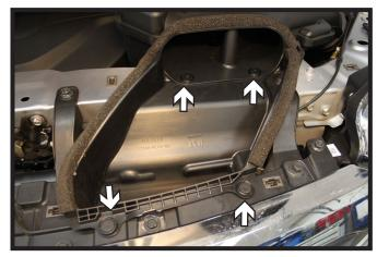
2. Remove the four (4) screws from the intake tube and set aside.
