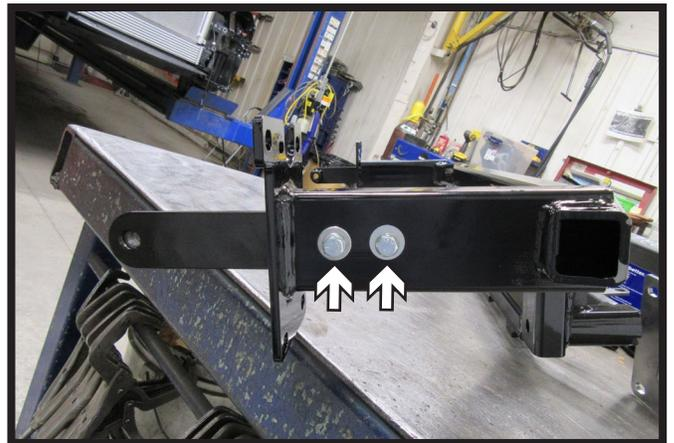
15. Place the baseplate on a flat surface and attach the support strap to the baseplate using two (2) 3/8" bolts. Make sure that the support strap is as straight as possible. Do not tighten fully. Do this for both sides of the baseplate.
