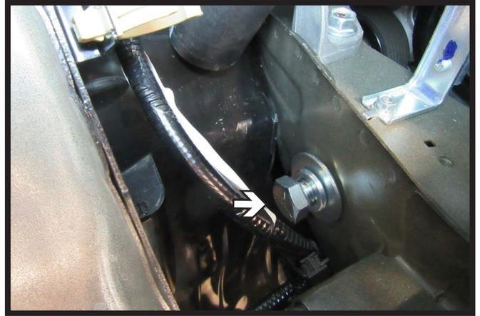
17. Start the 5/8" bolt with flat washer and lock washer. Do not tighten fully. Do this on both sides of the baseplate
