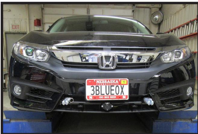
22. Hold the fascia as close to its original position, mark and trim the fascia around the convenience links and attachment tabs. Reinstall the headlights, fascia and fascia cover.
