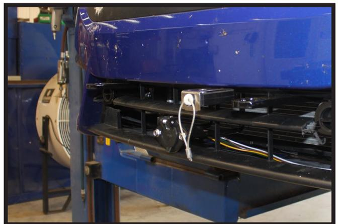
23. **Optional Breakaway:** In the desired location, drill a 1/4" hole thru the fascia lip. Install the breakaway to the fascia with the 1/4" hardware provided.
