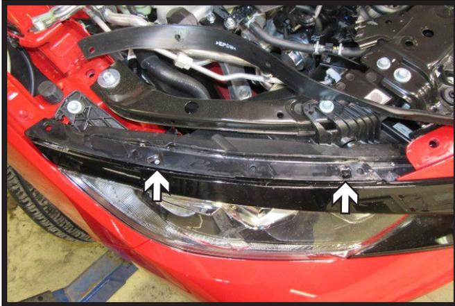
5. **2019 Models:** Remove the plastic piece above the head light using Phillips screw driver to press down on two (2) snaps. Do this on both sides of the vehicle.
