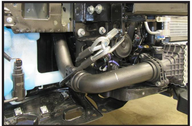
19. Reinstall turbo air coolant tube to the passenger side of the vehicle.
