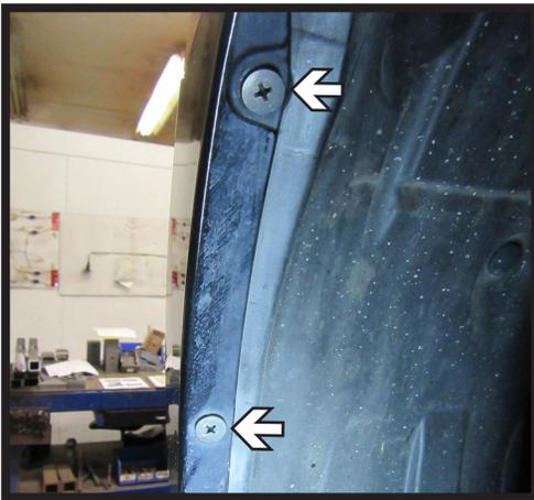
3. Using a Phillips screwdriver, remove the two (2) screws from the edge of the wheel well. Do this on both sides of the vehicle.
