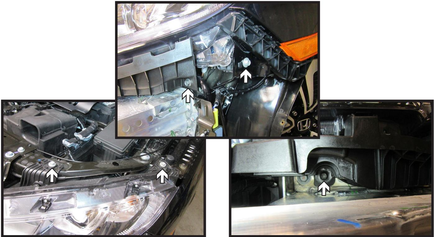
8. Using a 10MM socket, remove the five (5) screws from the headlight. Disconnect all electrical lines and set aside. Do this on both sides of the vehicle.
