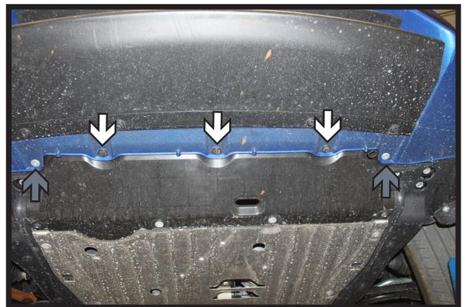
4. Using a 10MM socket, remove the bolt (gray) from the underside of the fascia. Then remove the two (2) push pins (left photo). Do this on both sides of the vehicle. Using a T30 Torx, remove the two (2) bolts towards the center (gray). Then remove the three (3) push pins (right photo).
