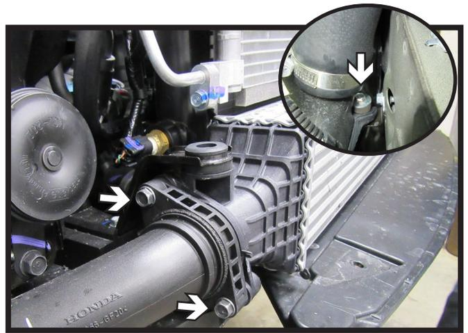
13. Using a 10MM socket remove the three (3) bolts attaching the turbo air coolant tube to the passenger side of the vehicle, two (2) in the front and one (1) in the back.
