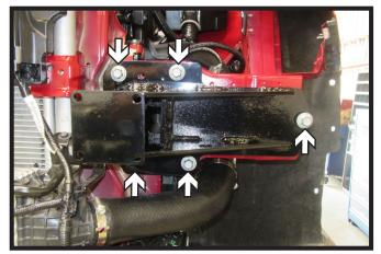
Hold the side plate in place and start the five (5) existing 14MM bolts. Do this on both sides of the vehicle.
