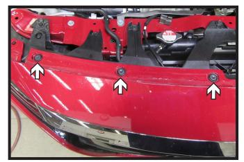
2. Remove the six (6) push pins from the top of the fascia, there are three (3) on each side of the vehicle.
