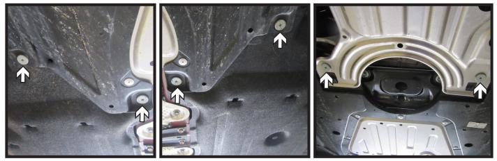
10. Using a Phillips screwdriver remove the six (6) screws from the underside of the vehicle.
