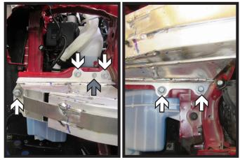
Using a 14MM socket, remove the five (5) bolts (white) from the bumper. Then using a 10MM socket, remove the one (1) bolt (gray) from the top of the bumper. Do this on both sides of the bumper. Remove bumper, it will not be reinstalled later.
