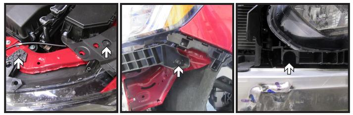
7. Using a 10MM socket, remove the four (4) bolts from the headlight. Remove the headlight and set aside to be reinstalled later. Do this on both sides of the vehicle.
