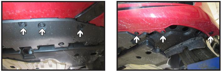
5. Remove the twelve (12) push pins from the underside of the vehicle, there are six (6) on each side. Remove fascia and unplug any electrical connections, set aside to be reinstalled later.
