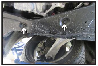
9. Remove the thirteen (13) push pins from the underside of the vehicle. There are seven (7) push pins on the passenger side and six (6) on the driver side of the vehicle.
