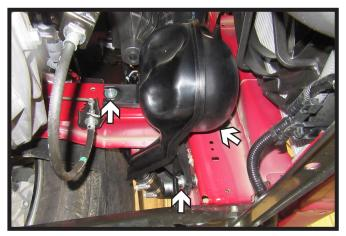
13. Using a 10MM socket, remove the three(3) bolts holding the air baffle on the driver side of the vehicle and let hang to allow access to the frame.
