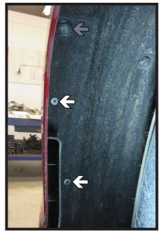
Using a Phillips screwdriver, remove the two (2) screws (white) from the wheel well. Then remove the one (1) push pin (gray). Do this on both sides of the vehicle.
