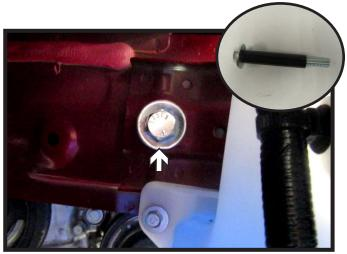
18. Place spacer tube on 1/2" x 4-1/2" bolt with flat washer (inset) and install bolt with second flat washer and nylon lock nut into back frame hole. Do this on both sides of the vehicle. Tighten front mounting strap bolts fully at this time.
