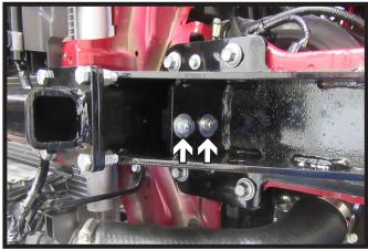
Slide mounting strap into place and start two (2) 3/8" x 1-1/4" bolts with flat washer and lock washer, leave loose. Do this on both sides of the vehicle.
