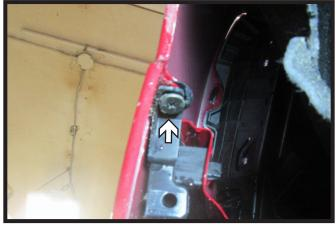
Pull back the wheel well liner and using a Phillips screwdriver, remove the one (1) screw. Do this on both sides of the vehicle.
