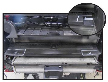
14. Using a utility knife trim both sides of the air dam as shown. Make sure to trim the extra area on the driver side of the vehicle (inset) to allow room for breakaway bracket.
