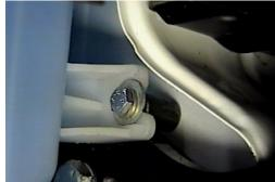
10. To reinstall windshield washer reservoir, it will be necessary to use spacer tube item 14 and item 15 for the front bolt. The upper bolt location will need to drilled. Reinstall remaining bolts.
