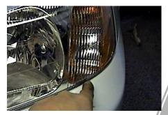
**6.** Just under head light assemblies is a push pin to remove, both sides. Pull fascia forward and set aside.
