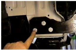
8. Remove the tow brackets with the 17MM socket, both sides. Hold baseplate to align with these holes and install items 3, 4 and 5, both sides. Tighten all bolts. Note: Use spacer plate, item 3, as needed, apply equally to each side. Be sure and use loctite on all bolts before tightening. Torque all bolts according to torque chart on General Instructions sheet.
