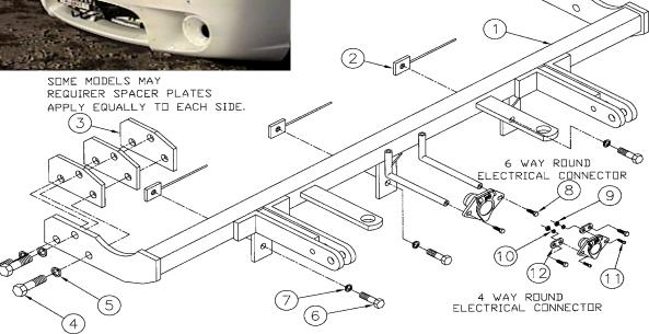
**IMPORTANT:** Use only genuine factory replacement parts on your Base Plate. Do not substitute homemade or nontypical parts. If a bolt is lost or in need of replacement, for your safety and the preservation of your Base Plate, be sure to use a replacement bolt of the same grade (Usually Grade 5, refer to parts list). Repair parts may be ordered through your nearest **Blue Ox** dealer or distributor.
