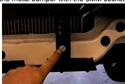
9. Using the baseplate as a template, drill the three remaining holes on cross member with the 13/32" drill bit. Insert item 2 into cross member openings to align with drilled holes, install items 6 and 7, and tighten. Be sure and use loctite on all bolts before tightening. Torque all bolts according to torque chart on General Instruction sheet.
