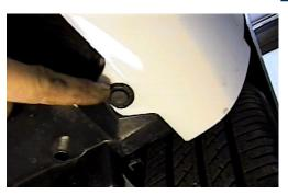
2. There are six phillips head push pins to remove from the bottom side of the fascia.
