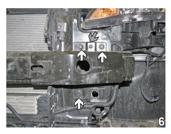
6. Using a 12MM socket, remove one (1) bolt below the bumper and the two (2) outside bolts above the bumper (white arrows). Using a 10MM socket, remove the middle bolt above the bumper (gray arrow). Do this to both sides of the vehicle. Set the bolts and bumper aside to be reinstalled later.
