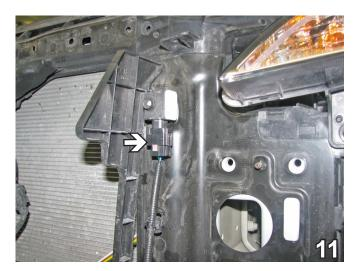
11. Unplug the air bag sensor by the corner of the headlight and move the electrical coax out of the way. It will be reinstalled later. Do this to both sides of the vehicle.
