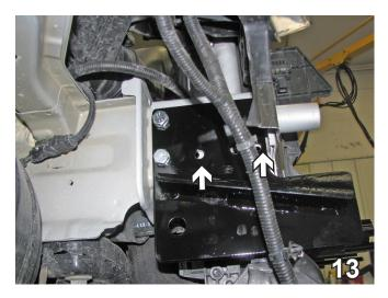
13. Using baseplate as a template, drill two (2) holes into frame rail with the 13/32" drill bit. Do this to both sides of the vehicle.
