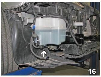
16. On the passenger side, reinstall the washer reservoir using the existing bolts. Reconnect the hose and electrical connection.
