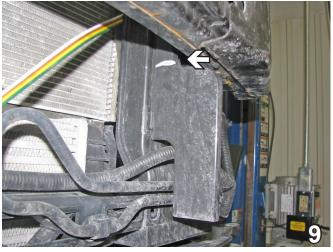
9. Using a utility knife, cut across the air dam flush with the bottom of the bumper and remove lower portion of air dam. Do this to both sides of the vehicle.
