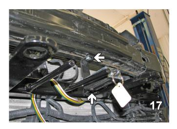
17. **Optional:** Drill a hole into the bottom of the bumper 3/4" from the front side and halfway between electrical rod and convenience link on the drivers side with a 9/32" drill bit. Fasten the bracket to the underside of the bumper with 1/4"-20 x 3/4" hex bolt and 1/4"-20 hex nut. Attach the breakaway to the bracket with a 1/4"-20 x 3/4" hex bolt and 1/4-20 hex nut.
