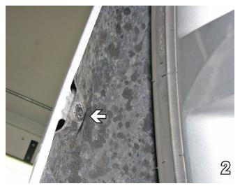
Using the 8MM socket, remove one (1) metric bolt from edge of fascia, just inside wheel well.
