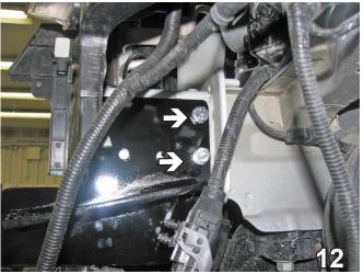
12. Slide the baseplate on to frame that will align with existing bolt holes, start two (2) 10MM-1.25 x 30MM bolts in the existing back holes with 10MM lock washers and 10MM flat washers. Be sure the baseplate is level with respect to the vehicle frame and tighten the bolts with the 17MM socket. Be sure to use Loctite Red on all bolts. Do this to both sides of the vehicle.
