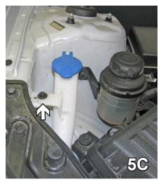
5. On the passenger side, disconnect the hose and electrical connection from the washer reservoir and plug the hose. Using the 10MM socket, remove three metric bolts from the washer reservoir. Remove washer reservoir. Set bolts and reservoir aside to be reinstalled later.
