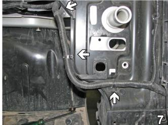
Remove the three (3) push pins holding the coax hose and move out of the way for baseplate installation. Do this to both sides of the vehicle. Set the push pins aside to be reinstalled later.
