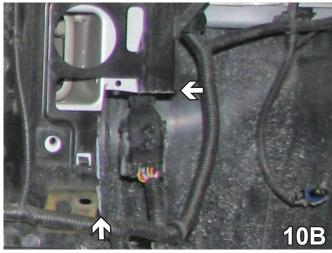
10. Using the reciprocating saw, make a horizontal cut in the frame webbing flush with the bottom of the bumper and straight up from the side of the frame (drivers side shown). Do this to both sides of the vehicle.
