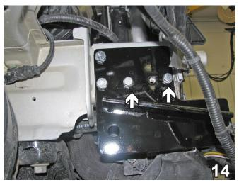
14. Insert 3/8"-16 nut plates through the frame end opening. Align to the lower outside two (2) drilled holes. Install 3/8"-16 x 1-1/4" hex bolts with 3/8" lock washers and tighten. Be sure to use Loctite Red on all bolts. Do this to both sides of the vehicle.
