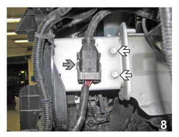
8. On the drivers side, pull out christmas tree plug from frame extension on the back side of electrical connector and pull electrical connection out of the way to install baseplate gray arrow). Remove the two metric bolts with the 14MM socket (white arrows). Do this to both sides. These bolts will not be used later.
