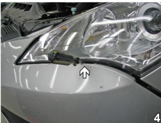
4. Lift up and pull the upper corners of fascia to the side to release from the tabs. Under the headlight use a flat screwdriver to lift up and pull out to unsnap. Do this to both sides of the vehicle. Pull fascia forward to remove. Set fascia aside carefully to be reinstalled later.
