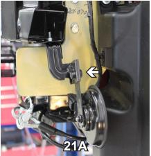
21. To reinstall the horn on driver's side, flatten the notch at the end of the horn bracket by tapping with a hammer (21A). Drill a 1/4" hole through the bottom of the metal bumper (21B). Insert 1/4"-20 x 3/4" hex bolt with 1/4"-20 hex flange whiz nut to attach horn bracket. Use existing bolt to attach horn to horn bracket (20C).
