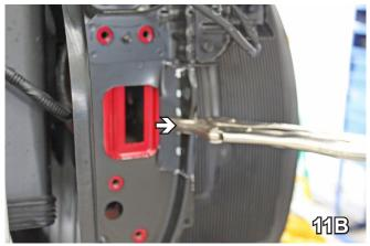
11. With reciprocating saw, cut into upper bumper guard (flush with metal brace) where indicated on 11A. The two (2) cuts will be 4-1/4" apart. After cuts have been made, with large vise grips, toggle the cut area back and forth until it breaks free (11B). Do this to both sides.
