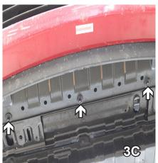
3. Under fascia, with Phillips screwdriver, remove two (2) push pins from each side (3A and 3B). With a 10MM socket, underneath the fascia, toward the middle, remove three (3) bolts (3C). Set push pins and bolts aside to be reinstalled later.
