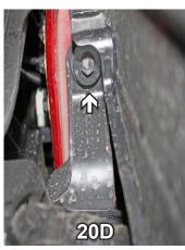
20. Trimming of the air baffle is required before reinstallation. With a utility knife, trim the lower bolt tab off of the air baffle as shown in 20A. A picture of the completed trimming is shown in 20B. Reinstall the air baffle on the driver's side using 6MM-1.00 x 45MM hex bolt with 3/8" flat washer and 3/8" lock washer for top bolt hole (20C) and existing bolt on the bottom side of the air baffle (20D). Tighten bolts with Loctite Red.
