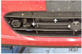
24. In order to accommodate attachment tabs through the fascia of the vehicle, with a utility knife, trim middle piece of fascia referenced in 24A. Do this to both sides of the vehicle. Picture of completed trimming shown in 24B.
