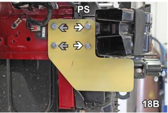
18. Using a 13/32" drill bit, drill remaining 3 holes for mounting baseplate. Do this to both sides. Insert 3/8"-16 x 1-1/4" hext bolt, 3/8" lock washer, 3/8" flat washer and 1/4"-20 x 1" x 1" nut plate into each drilled hole.
