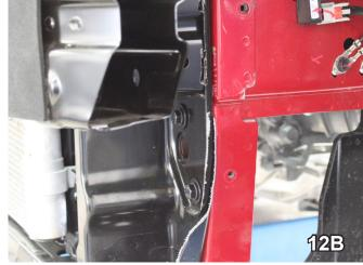
12. With reciprocating saw, cut lower bumper guard (flush with metal brace) where indicated on 12A. Do this to both sides. An example of the completed trimming is referenced in 12B. Reinstall bumper using existing bolts.
