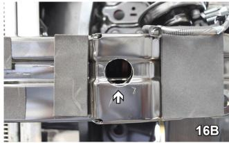
16. On the front of the bumper, toward the outer edge of the bumper, with a 1-1/4" hole saw, cut through the front two (2) layers of the metal bumper (1st layer cut is shown in 16A - 2nd layer cut is shown in 16B). Do this to both sides. Nut plates will be inserted through these holes at a later point in the instructions.
