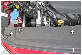
1. To remove radiator cover, with 10MM socket, remove four (4) bolts (white arrows - two (2) per side). To remove additional piece connected to the radiator cover, push in on the push pins and lift up to remove (gray arrows). Set radiator cover in its entirety along with bolts and push pins aside to be reinstalled later.
