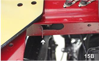
15. Underneath the framerail, with a reciprocating saw, make two (2) horizontal cuts as shown in 15A (between 1" - 1-1/2" long). With a vise grip, bend the metal between the cuts to widen the opening underneath the frame rail (15B). Do this to both sides. These openings will be used to insert the nut plates at a later point in the instructions.
