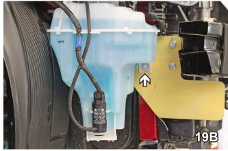
19. Reinstall washer reservoir on passenger's side using existing bolts in the back of the reservoir (19A) and on the side of the reservoir, use 6MM-1.00 30MM hex bolt into existing hole with 3/8" flat washer and 3/8" lock washer (19B). Tighten bolts with Loctite Red. Reattach fluid lines and electrical connections.
