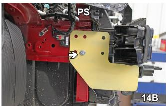
14. When mounting baseplate to the vehicle, use the existing holes on side rails to align and keep level as shown above. On driver's side, insert 6MM-1.00 x 45MM hex bolt into existing hole as shown in 14A with 3/8" flat washer and 3/8" lock washer. On passenger's side, insert 6MM-1.00 x 30MM hex bolt into existing hole as shown in 14B with 3/8" flat washer and 3/8" lock washer. (*Baseplate painted yellow for illustration. Actual baseplate will be powder-coat black.*)
