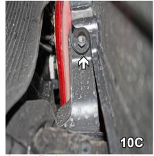
10. To remove air baffle on driver's side only, remove push pin on front of air baffle (10A - gray arrow) and with a 10MM socket, remove two bolts at the front of the air baffle as seen in 10A - white arrow. Disconnect hose from air baffle as shown in picture 10B. Underneath fascia in front of the tire, with 10MM socket, remove bolt shown in picture 10C. Set bolts, push pin, and air baffle aside to be reinstalled later.
